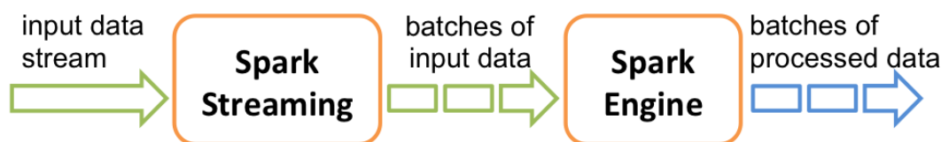
Figure 2. Schematic of stream processing in Spark.
