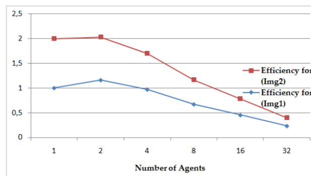
Figure 18. Efficiency of DFCM classification depending on the number of AVPEs and with initial class centers (c_1, c_2, c_3) = (1.1, 2.5, 3.8) for Img1, and (c_1, c_2, c_3, c_4, c_5) = (1.5, 2.2, 3.8, 5.2, 8.6) for Img2.
