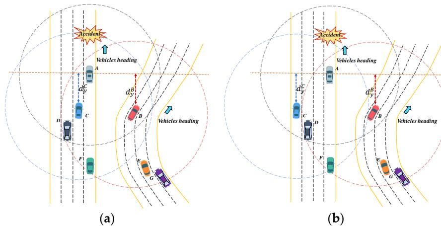
**Figure 7.** Example of broadcast dissemination process using Equation (5): (a) when A and B nodes are located in the same wireless range; (b) when A and B nodes are out of one another's wireless range.
