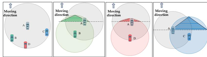
Figure 8. Selection of relay vehicle using the proposed algorithm.
