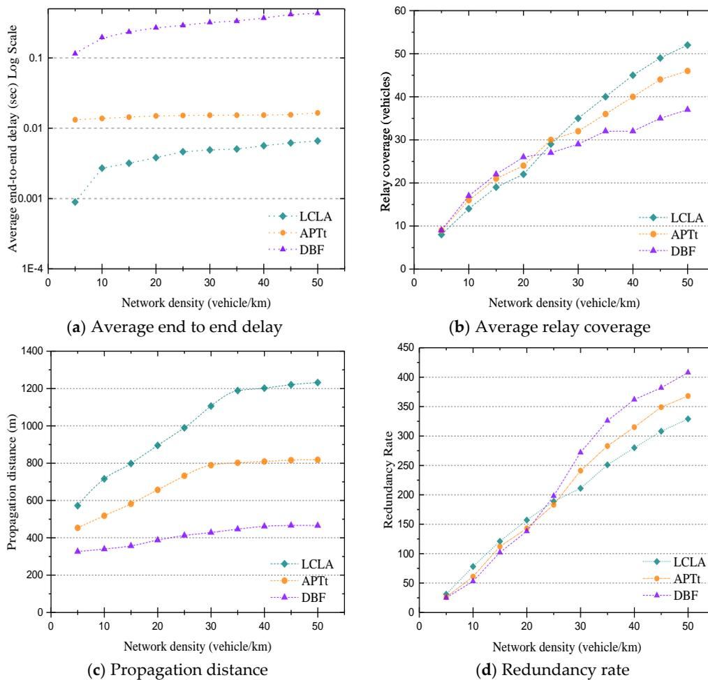
**Figure 11.** The results of proposed algorithm for a multilane highway scenario. The figures illustrated in these graphs represents an average value of corresponding performance metric for different vehicle number.
