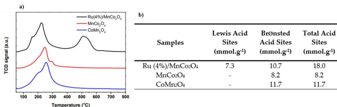
**Figure 4.** (a) NH<sub>3</sub>-TPD and (b) summarized data obtained from NH<sub>3</sub>-TPD for CoMn<sub>2</sub>O<sub>4</sub>, MnCo<sub>2</sub>O<sub>4</sub> and Ru/MnCo<sub>2</sub>O<sub>4</sub> catalyst (reproduced from [81] with permission from the Royal Society of Chemistry, copyright 2017).
