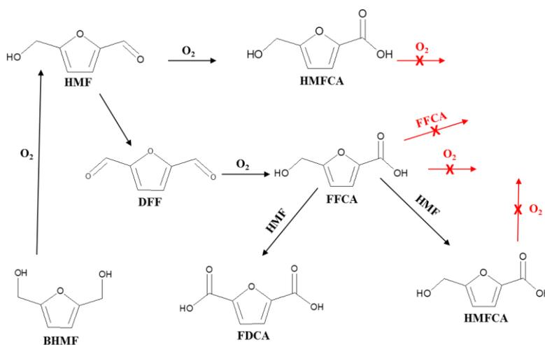
**Scheme 6.** Reaction pathways for HMF oxidation over Pd-Au/TiO<sub>2</sub> catalyst (reproduced from [73] with permission from Elsevier, copyright 2015).
