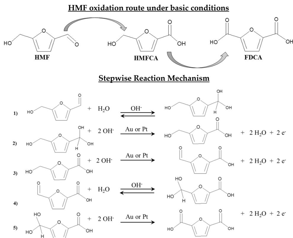
**Scheme 4.** Expanded reaction pathway of HMF oxidation in basic ( $\text{OH}^-$ ) media over Au or Pt catalysts (reproduced from [48,49] with permission from Royal Society of Chemistry & Elsevier, copyright 2012 and 2014).
