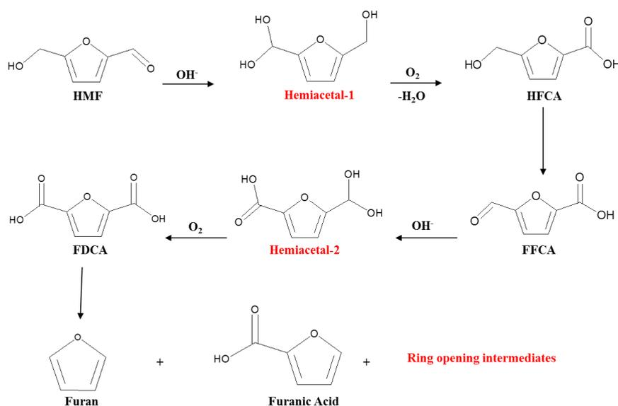
**Scheme 3.** Reaction mechanisms for aerial oxidation of aqueous HMF over  $\text{CeO}_2$  supported Au catalysts (reproduced from [36] with permission from Wiley-VCH, copyright 2009).
