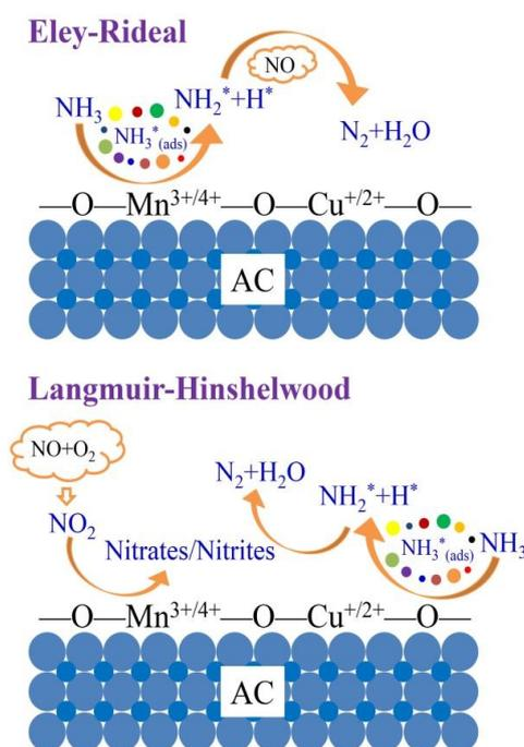
Figure 10. NO removal mechanism of the  $\text{MnO}_x\text{-Cu/AC}$  catalyst.
