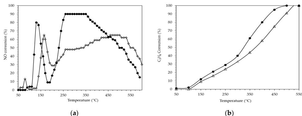
**Figure 10.** NO and  $C_3H_8$  conversion in the reaction  $C_3H_8$ -SCR-NO. (a) NO conversion with (●) 0.1PtAg/AW and (◇) 2Ag/AW; (b)  $C_3H_8$  Conversion with (●) 0.1PtAg/AW and (△) 2Ag/AW catalysts. Inlet gas composition: 500 ppm NO, 625 ppm  $C_3H_8$ , 200 ppm CO, 660 ppm  $H_2$ , 2 vol.%  $O_2$ ,  $N_2$  balance; GHSV = 128,000  $h^{-1}$ .
