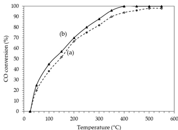
**Figure 11.** CO conversion of catalysts: (a) 2Ag/AW and (b) 0.1PtAg/AW. Inlet gas composition: 500 ppm NO, 625 ppm  $C_3H_8$ , 200 ppm CO, 660 ppm  $H_2$ , 2 vol.%  $O_2$ ,  $N_2$  balance; GHSV = 128,000  $h^{-1}$ .
