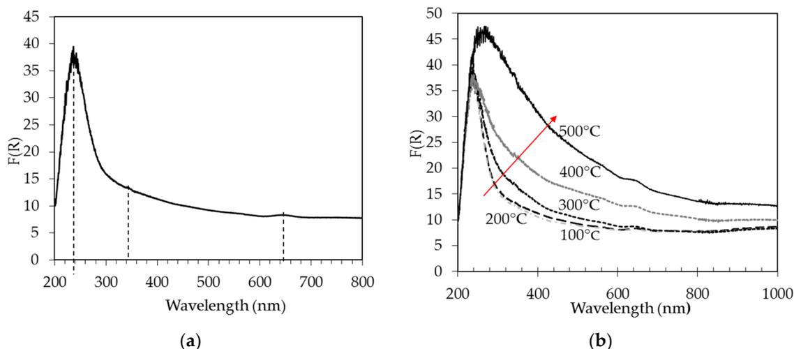
**Figure 5.** In situ UV-Vis spectrum of: (a) 0.4Pt/AW catalyst calcined at 500 °C; (b) 0.4Pt/AW catalyst during the reduction process with 5 vol.% H<sub>2</sub>/N<sub>2</sub>, 0.5 cm<sup>3</sup>/s.
