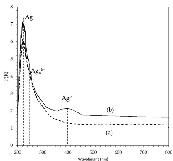
**Figure 4.** Ex situ UV–Vis spectra of the catalysts: (a) Calcined 2Ag/AW; (b) 2Ag/AW after H<sub>2</sub> reduction in a flow of H<sub>2</sub> (30 cm<sup>3</sup>/min) at 500 °C for 2 h (spectrum taken immediately after reduction in H<sub>2</sub>).
