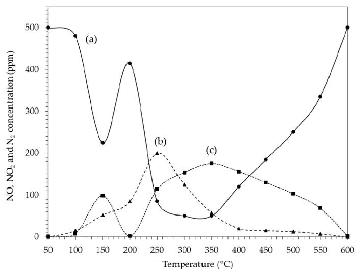
**Figure 12.** Composition of (a) NO; (b) NO<sub>2</sub> and (c) N<sub>2</sub> (calculated) in the microreactor as a function of temperature during the C<sub>3</sub>H<sub>8</sub>-SCR-NO with the catalyst 0.1PtAg/AW in the presence of H<sub>2</sub>. Inlet gas composition: 500 ppm NO, 625 ppm C<sub>3</sub>H<sub>8</sub>, 200 ppm CO, 660 ppm H<sub>2</sub>, 2vol.% O<sub>2</sub>, N<sub>2</sub> balance; GHSV = 128,000 h<sup>-1</sup>.
