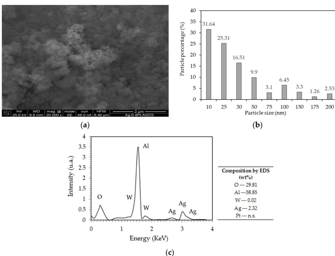
**Figure 3.** Morphological and chemical composition of the catalyst 0.4PtAg/AW calcined at 500 °C. (a) SEM micrograph; (b) The distribution of particle diameters; (c) EDS analysis of the spherical cumulus zone where Pt cannot be analyzed due to its low concentration.
