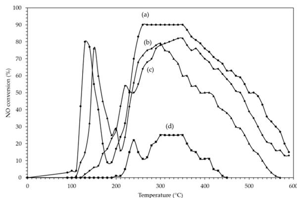
**Figure 9.** Bimetallic catalyst of PtAg for the  $C_3H_8$ -SCR-NO: (a) 0.1PtAg/AW; (b) 0.25PtAg/AW; (c) 0.4PtAg/AW; (d) 1PtAg/AW in the presence of  $H_2$ . Inlet gas composition: 500 ppm NO, 625 ppm  $C_3H_8$ , 200 ppm CO, 660 ppm  $H_2$ , 2 wt%  $O_2$ ,  $N_2$  balance; GHSV = 128,000  $h^{-1}$ .
