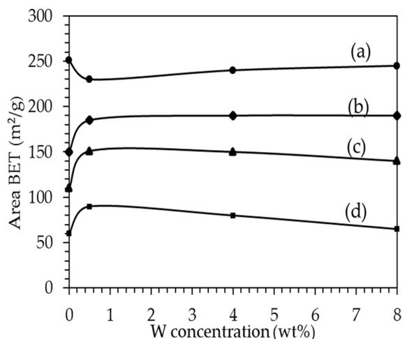
**Figure A1.** BET area against W concentration (in wt%W) named  $\text{Al}_2\text{O}_3\text{-WO}_x$ , when the calcination temperature increased: (a) 500 °C; (b) 650 °C; (c) 800 °C; (d) 950 °C for 6 h.
