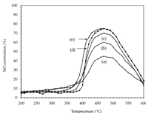
**Figure 8.**  $C_3H_8$ -SCR- $NO_x$  from (a) 1PtAg/AW catalyst; (b) 0.4PtAg/AW catalyst; (c) 0.25PtAg/AW catalyst; (d) 2Ag/AW catalyst; (e) 0.1PtAg/AW catalyst. Inlet gas composition: 500 ppm NO, 625 ppm  $C_3H_8$ , 200 ppm CO, 2 vol.%  $O_2$ ,  $N_2$  balance; GHSV = 128,000  $h^{-1}$ .
