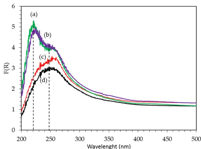
**Figure 6.** Ex situ UV-Vis spectra of the PtAg/AW catalysts calcined at 500 °C when the Pt concentration changed from 0.1 to 1 wt% on Al<sub>2</sub>O<sub>3</sub>-WO<sub>x</sub> catalysts. (a) 1PtAg/AW; (b) 0.4PtAg/AW; (c) 0.25PtAg/AW; and (d) 0.1PtAg/AW.
