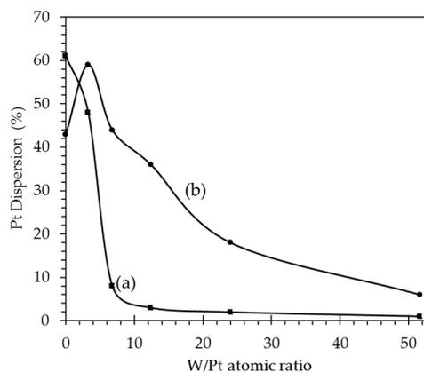
**Figure A2.** Dispersion of Pt in Pt/AW catalysts increasing the W/Pt atomic ratio when the reduction temperature in  $\text{H}_2$  increased from (a) 500 to (b) 800 °C (for 4 h).
