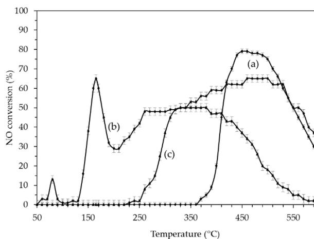
**Figure 7.** C<sub>3</sub>H<sub>8</sub>-SCR-NO<sub>x</sub> from (a) 2Ag/AW catalyst in the absence of H<sub>2</sub>; (b) 2Ag/AW catalyst in the presence of H<sub>2</sub>; (c) 0.4Pt/AW catalyst in the presence of H<sub>2</sub>. Inlet gas composition: 500 ppm NO, 625 ppm C<sub>3</sub>H<sub>8</sub>, 200 ppm CO, 660 ppm H<sub>2</sub>, 2 vol.% O<sub>2</sub>, N<sub>2</sub> balance; GHSV = 128,000 h<sup>-1</sup>.
