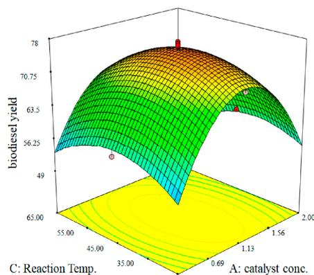
**Figure 2.** Surface response plot of first order interaction term showing significant impact on yield of biodiesel produced by chemical transesterification.
