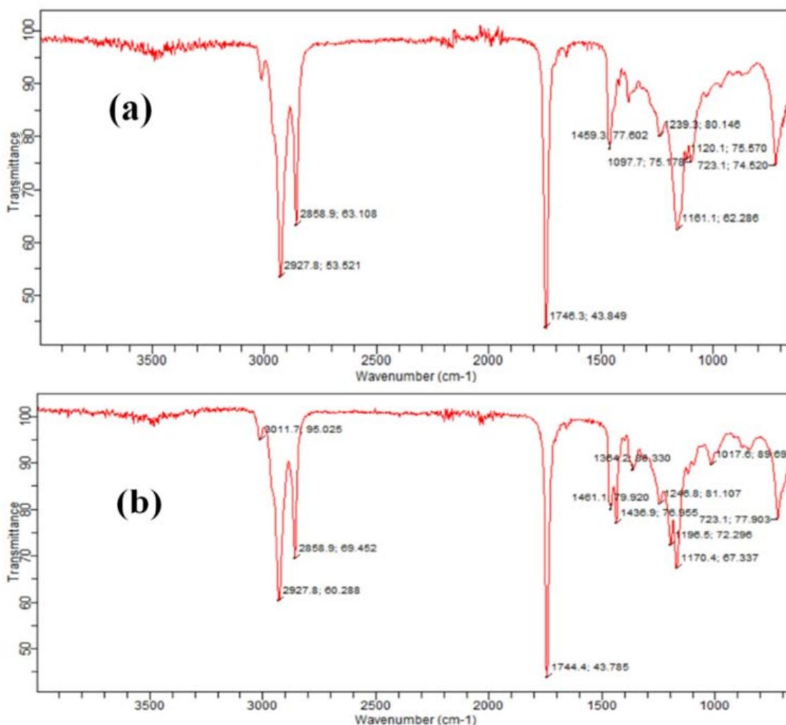
**Figure 4.** FTIR Spectrum (a) *Spirogyra oil* (b) *Spirogyra oil*-based biodiesel.
