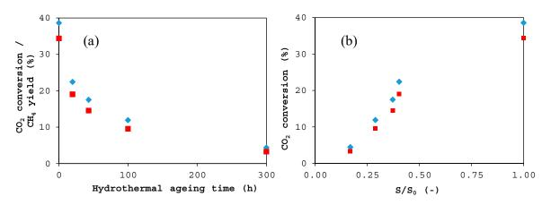
**Figure 2.** Catalyst activity measurements at 350 °C of fresh and post mortem samples aged at 600 °C in hydrothermal conditions (H<sub>2</sub>:H<sub>2</sub>O = 0.26) as a function of hydrothermal ageing time (**a**) and relative metallic surface (**b**)  $\blacklozenge$ : CO<sub>2</sub> conversion  $\blacksquare$ : CH<sub>4</sub> yield.
