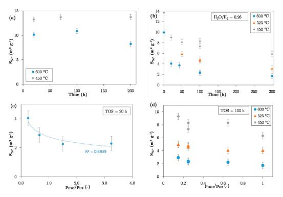
**Figure 3.** (a) Effect of temperature on metal particle sintering in reductive atmosphere  $H_2:N_2$ ; (b) effect of temperature on metal particle sintering under  $H_2:H_2O$  atmosphere, with a  $H_2O$  to  $H_2$  ratio of 0.26; effect of  $H_2O$  to  $H_2$  ratio on metal particle sintering (c) for 20 h at 600 °C and (d) for 100 h at 450, 525 and 600 °C.
