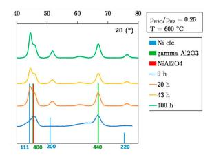
**Figure 5.** XRD pattern of the commercial Ni/Al<sub>2</sub>O<sub>3</sub> catalyst aged in hydrothermal conditions at 600 °C with a H<sub>2</sub>O to H<sub>2</sub> molar ratio of 0.26.
