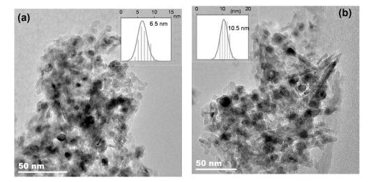
**Figure 6.** TEM images and nickel particle size distribution for the catalyst samples aged for 20 h (**a**) and 100 h (**b**) in hydrothermal conditions at 600 °C with a  $H_2O$  to  $H_2$  ratio of 0.26.
