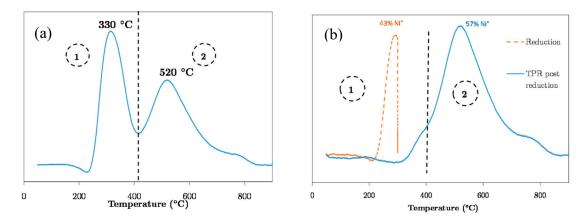
**Figure 1.** (a) H<sub>2</sub>-TPR of the fresh commercial catalyst Ni/Al<sub>2</sub>O<sub>3</sub>; (b) Activation procedure at 300  $^{\circ}$ C followed by a H<sub>2</sub>-TPR from 50 until 900  $^{\circ}$ C.
