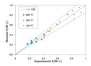
**Figure 8.** Parity plot of the experimental and modeled metallic surface area up to 300 h aging within 15% error at 450, 525 and 600 °C for a  $H_2O:H_2$  ratio ranging from 0 to 3.2.
