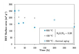
**Figure 4.** Evolution of the specific surface area with time at 450 °C and 600 °C in thermal and hydrothermal aging.
