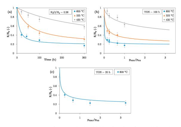
**Figure 7.** Comparison of experimental and modeled loss of metallic surface area (**a**) for 300 h hydrothermal aging at 450, 525 and 600 °C under H<sub>2</sub>:H<sub>2</sub>O atmosphere, with a H<sub>2</sub>O to H<sub>2</sub> ratio of 0.26; for several H<sub>2</sub>O to H<sub>2</sub> ratios (**b**) for 100 h at 450, 525 and 600 °C and (**c**) for 20 h at 600 °C.
