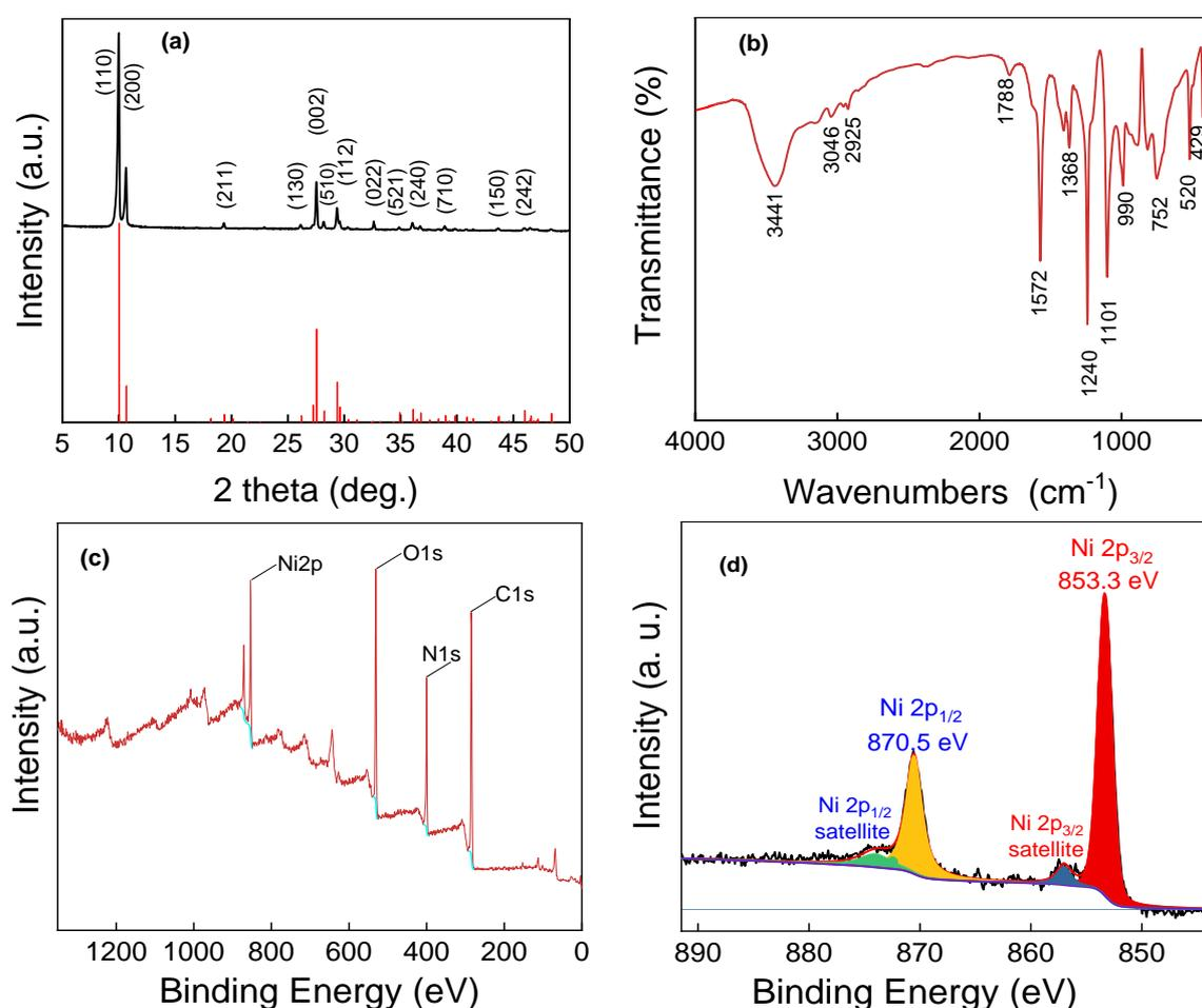
**Figure 2.** (a) XRD pattern, (b) FT-IR spectrum, (c) XPS survey spectrum and (d) Ni 2p XPS high-resolution spectra of the Ni(DMG)<sub>2</sub> complex.
