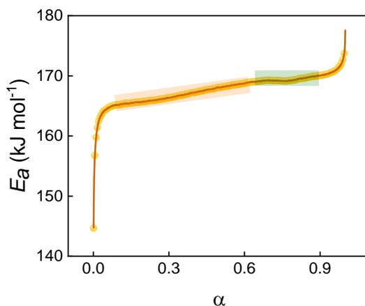
Figure 6.  $E_a$ - $\alpha$  curve for the thermal decomposition of Ni(DMG)<sub>2</sub> complex.
