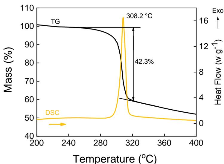
Figure 3. TG-DSC curves of the  $\text{Ni}(\text{DMG})_2$  complex.
