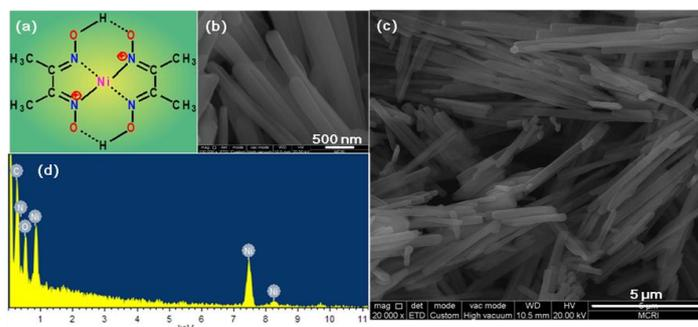
**Figure 1.** (a) Chemical structure of the bis-(dimethylglyoximate) nickel(II) complex ( $\text{Ni}(\text{DMG})_2$ ) molecule. (b,c) SEM images and (d) EDS spectra of the  $\text{Ni}(\text{DMG})_2$  complex.
