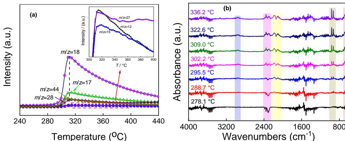
**Figure 4.** (a) MS and (b) FT-IR spectra of the evolved products released during the decomposition of Ni(DMG)<sub>2</sub> complex at different temperatures.
