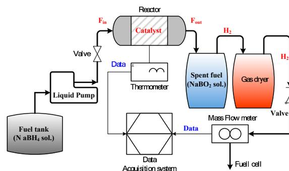
Figure 8. High-mobility hydrogen production system architecture diagram.
