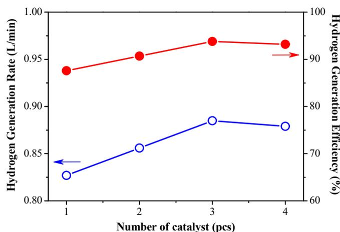
Figure 2. Effect of increasing catalyst dosage on hydrogen production efficiency (1). (Fuel 2g/min).
