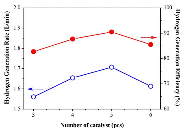
Figure 4. Effect of increasing catalyst dosage on hydrogen production efficiency (3). (Fuel 4g/min).
