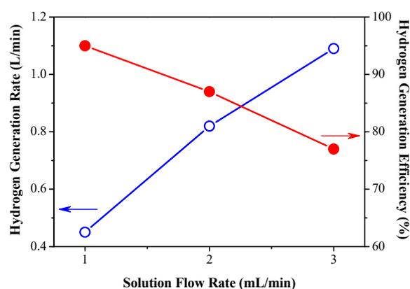
**Figure 1.** Effect of fuel feed flow on hydrogen production efficiency.
