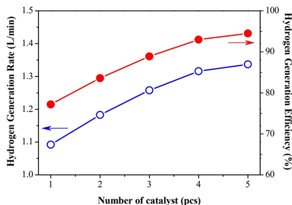
Figure 3. Effect of increasing catalyst dosage on hydrogen production efficiency (2). (Fuel 3g/min).
