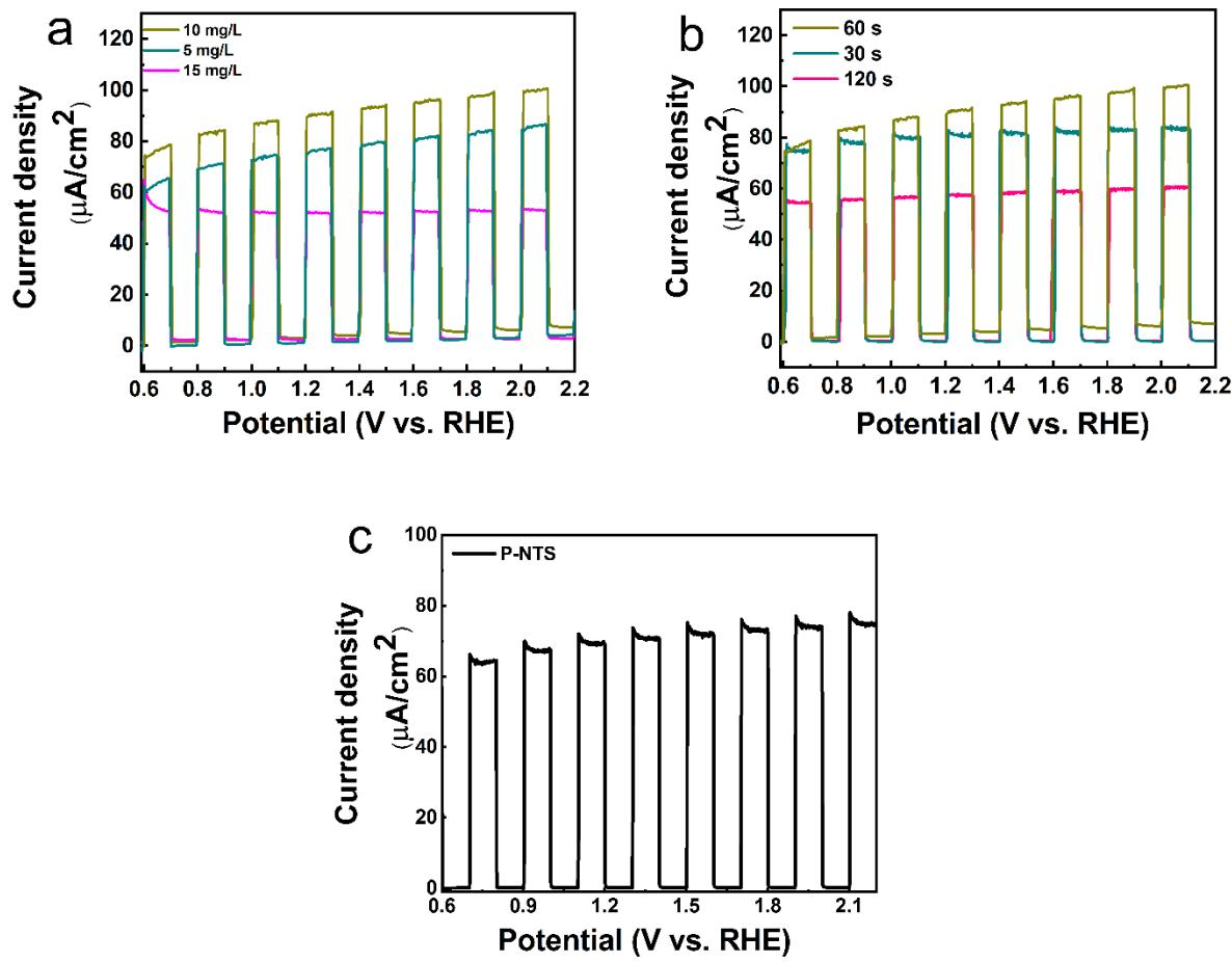
**Figure S2.** Photoelectrochemical response of synthesized samples measured under 1 sun illumination (100 mWc/m<sup>2</sup>-AM1.5 G) in 1 M NaOH solution at (a) different concentration of cyanographene, (b) different electrodeposition time, and (c) pure NTs.
