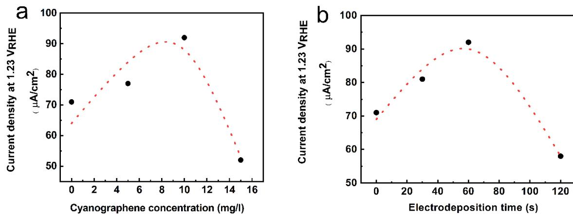
**Figure S1.** The effect of (a) cyanographene concentration and (b) electrodeposition time on the PEC-WS.
