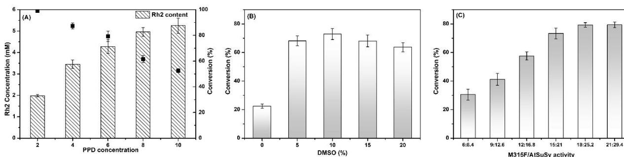
**Figure 4.** Optimization of the conditions for co-immobilized M315F and *AtSuSy* coupled reactions. Effect of PPD concentration on the Rh2 production by co-immobilized M315F and *AtSuSy* catalyzed reactions (A), conversion yield (■) was recorded. Effect of co-solvent DMSO on the yield of Rh2 by co-immobilized M315F and *AtSuSy* catalyzed reactions (B), and influence of different co-immobilized M315F and *AtSuSy* usage on the glycosylation reaction for Rh2 formation (C).
