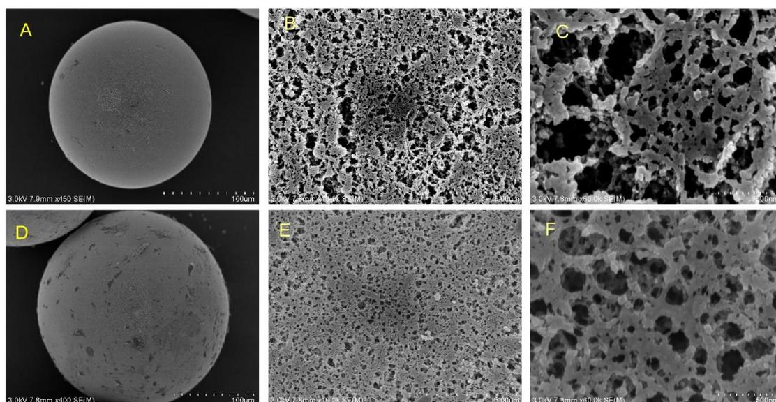
**Figure 2.** SEM images of resin heterofunctional resin (A–C) and resin immobilized with M315F/*AtSuSy* (D–F).
