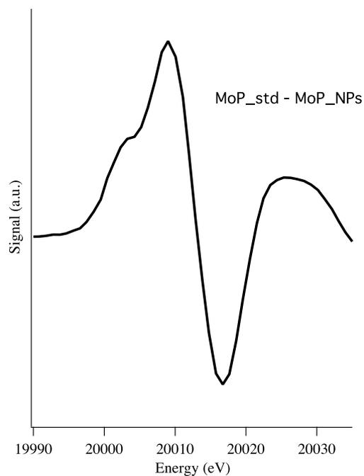
**Figure S2: XANES difference between crystalline MoP and as-prepared colloidal nanoparticles.**
