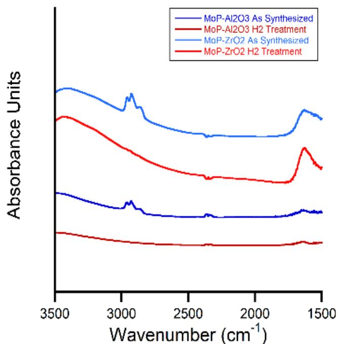
**Figure S1: C-H stretching region of the ex-situ IR spectra for supported MoP catalysts with the highest and lowest loading of MoP, showing the removal of ligands after hydrogen reduction treatment (450°C, 1 hour)**
