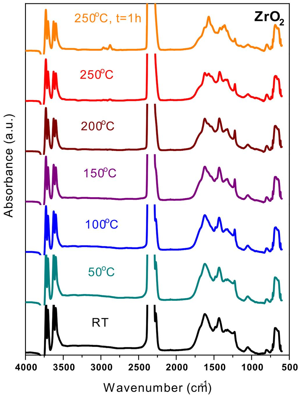
Figure S9: TPSR-DRIFTS full spectrum for  $\text{ZrO}_2$
