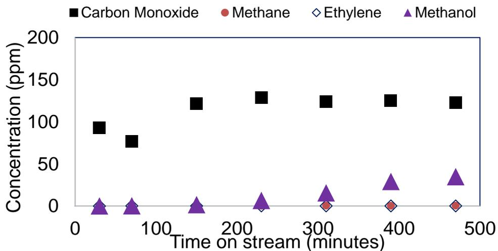
Figure S7: Activity of ZrO<sub>2</sub> support during CO<sub>2</sub> hydrogenation. Test conditions: CO<sub>2</sub> hydrogenation, 40 bar, 250°C, H<sub>2</sub>/CO<sub>2</sub>=3
