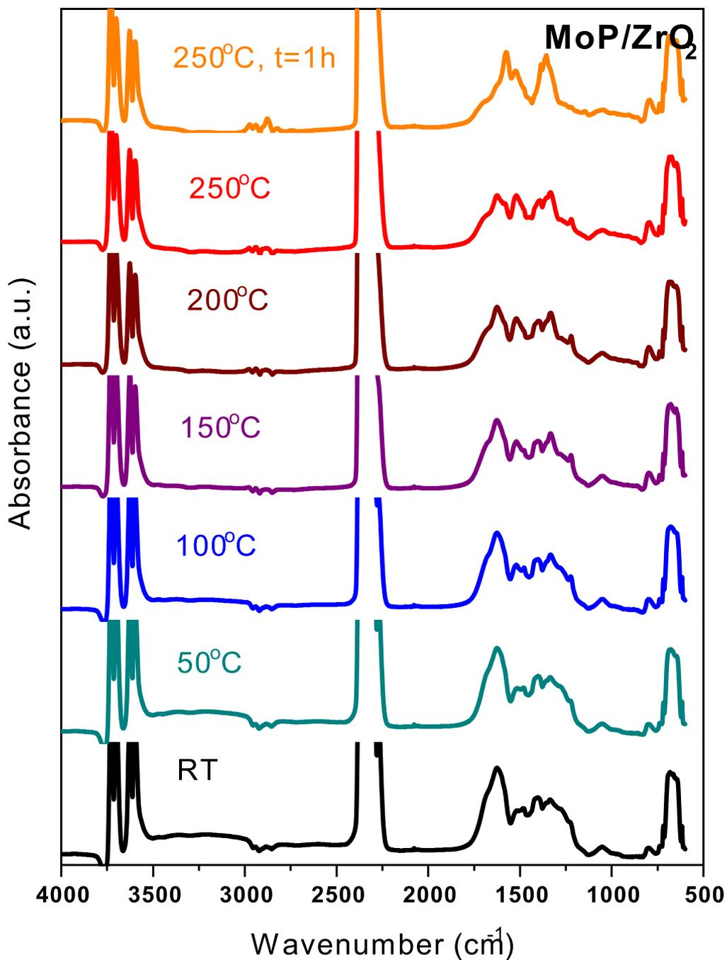
Figure S8: TPSR-DRIFTS full spectrum for MoP/ZrO<sub>2</sub>. Spectra were normalized to initial room temperature background taken under vacuum which is why the TOP ligands (see Figure S1) can be seen as negative peaks in the C-H stretching region (ligands were removed with the reduction treatment prior to TPSR) until higher temperatures when the formates begin to form and associated C-H stretching bands become dominant.
