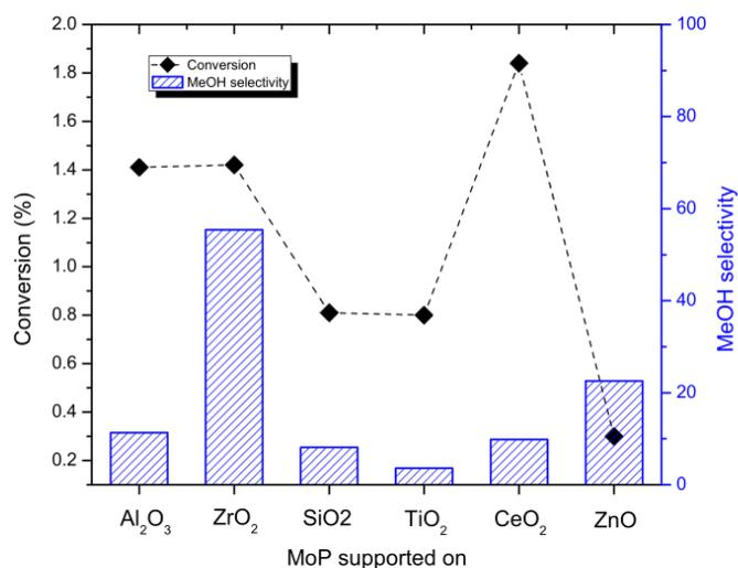
**Figure S5: Conversion and methanol selectivity of MoP nanoparticle catalysts on various supports during CO<sub>2</sub> hydrogenation. Test conditions: CO<sub>2</sub> hydrogenation, 40 bar, 250°C, H<sub>2</sub>/CO<sub>2</sub>=3, Conversion=0.3-1.8%. Data shown were collected after 7 hours on stream.**
