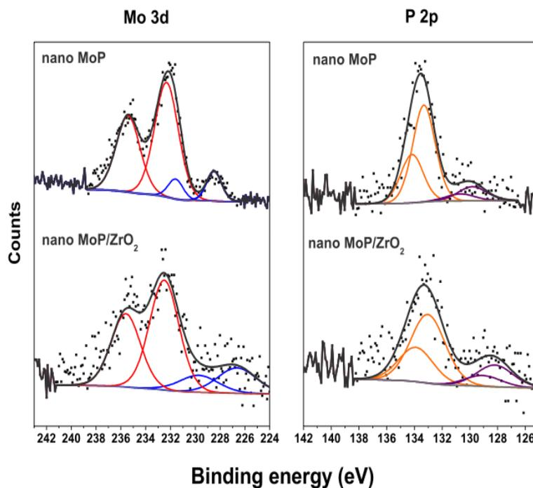
Figure S6: X-ray Photoelectron Spectroscopy (XPS) of air exposed unsupported and zirconia supported MoP nanoparticles
