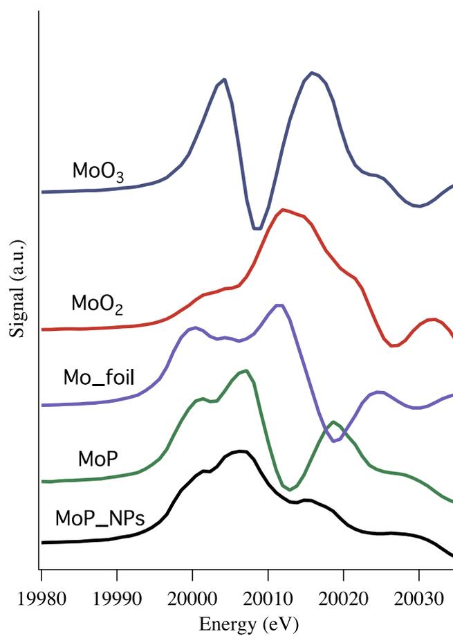
**Figure S3: First derivative of the XANES region of the Mo K-edge for different standards and as prepared Mo NPs at room temperature.**
