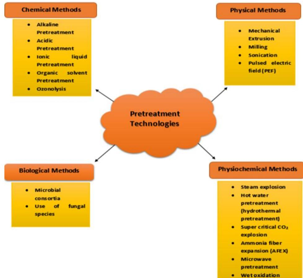
**Figure 4.** Flowchart of different pretreatment technologies.
