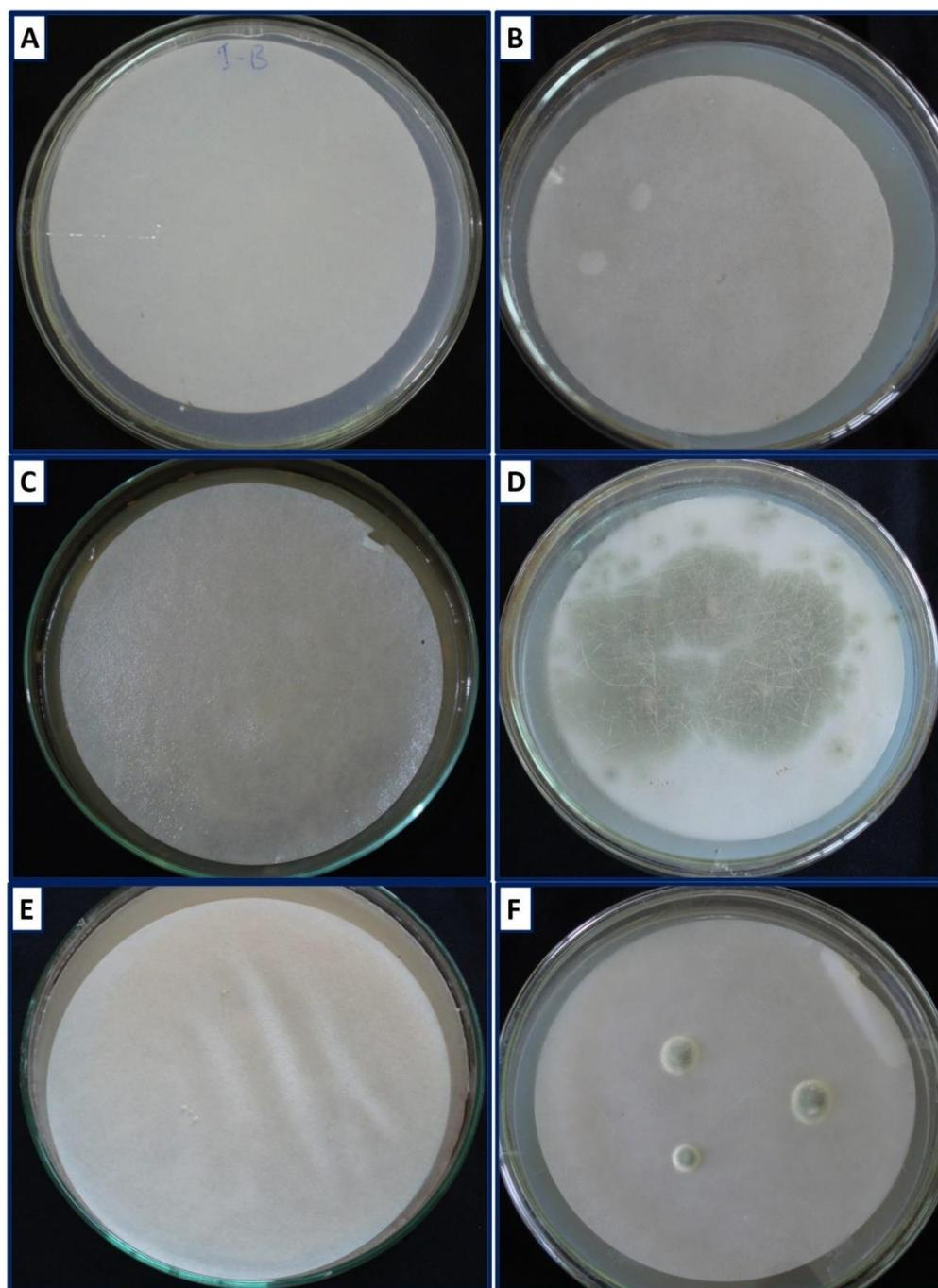
**Figure 3.** Photographic images for Whatman filter paper without any treatment (A), treated with  $80 \mu\text{g mL}^{-1}$  without microbial inoculation (B), untreated filter paper inoculated with *B. subtilis* B3 and *P. chrysogenum* F9 (C,D respectively), and treated filter paper inoculated with *B. subtilis* B3 and *P. chrysogenum* F9 after 21 days of aging (E,F, respectively).
