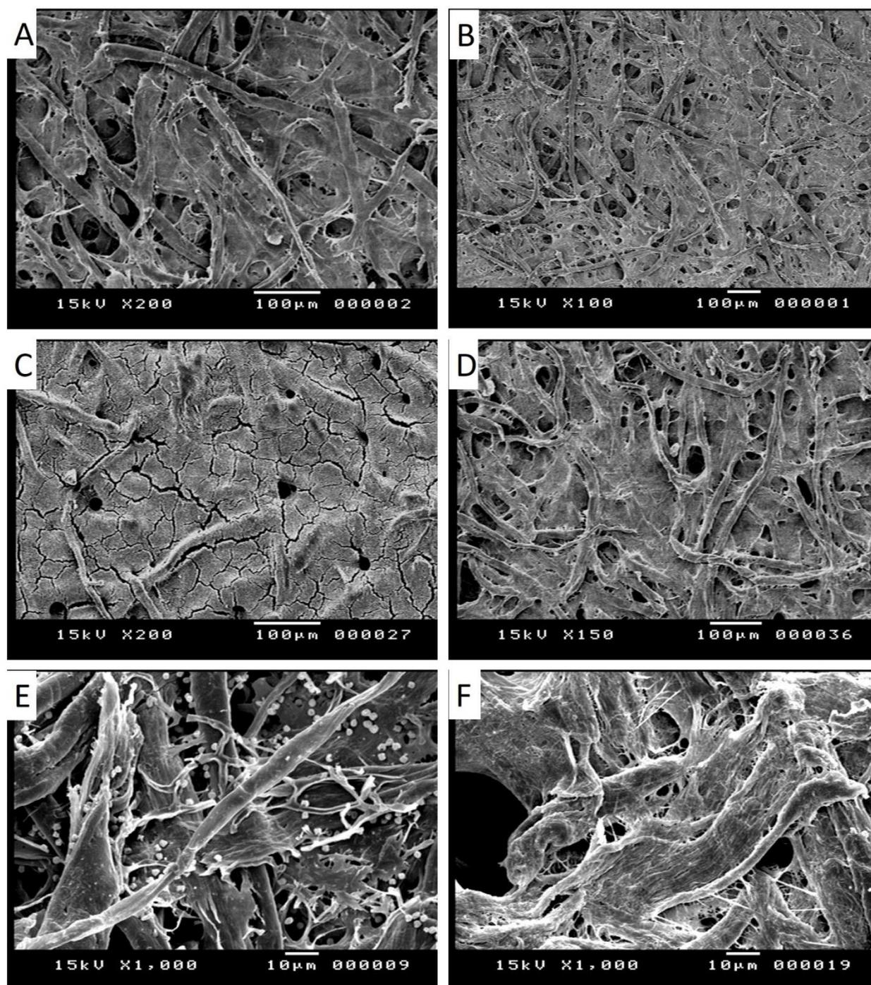
**Figure 5.** Scanning electron microscope (SEM) analysis of treated/untreated filter paper in the presence/absence of *B. subtilis* B3 and *P. chrysogenum* F9 after 21 aging days. (A) is the reference sample; (B) is negative control; (C) is untreated filter paper inoculated with *B. subtilis* B3; (D) is treated filter paper inoculated with *B. subtilis* B3; (E) is untreated filter paper inoculated with *P. chrysogenum* F9, and (F) is the treated filter paper inoculated with *P. chrysogenum* F9.
