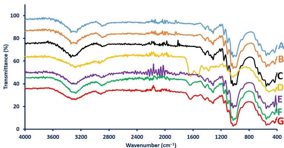
**Figure 4.** ATR-FTIR of treated/untreated filter paper in presence/absence of microbial inoculations after 21 aging days. A is reference sample; B is negative control; C is treated filter paper without microbial inoculation; D is untreated filter paper inoculated with *B. subtilis*; E is treated filter paper inoculated with *B. subtilis*; F is untreated filter paper inoculated with *P. chrysogenum*, and G is the treated filter paper inoculated with *P. chrysogenum*.
