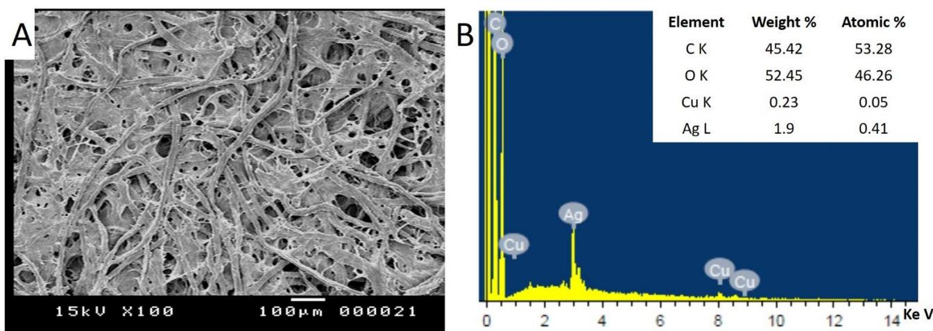
**Figure 2.** (A) SEM image of treated Whatman filter paper without microbial inoculation; (B) EDX profile exhibiting the chemical composition of treated filter paper.
