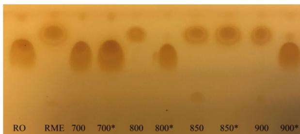
**Figure 3.** Reaction products of rapeseed oil transesterification with methanol using dolomite heated at different temperatures: the figures correspond to the temperature at which the dolomite was heated, RO—rapeseed oil, RME—methyl esters of rapeseed oil.
