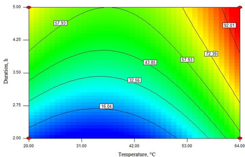
**Figure 4.** Response surface contour plot for the interaction between the process duration and the temperature for the ester yield when the catalyst amount is 6 wt% and the methanol-to-oil ratio is 12:1.
