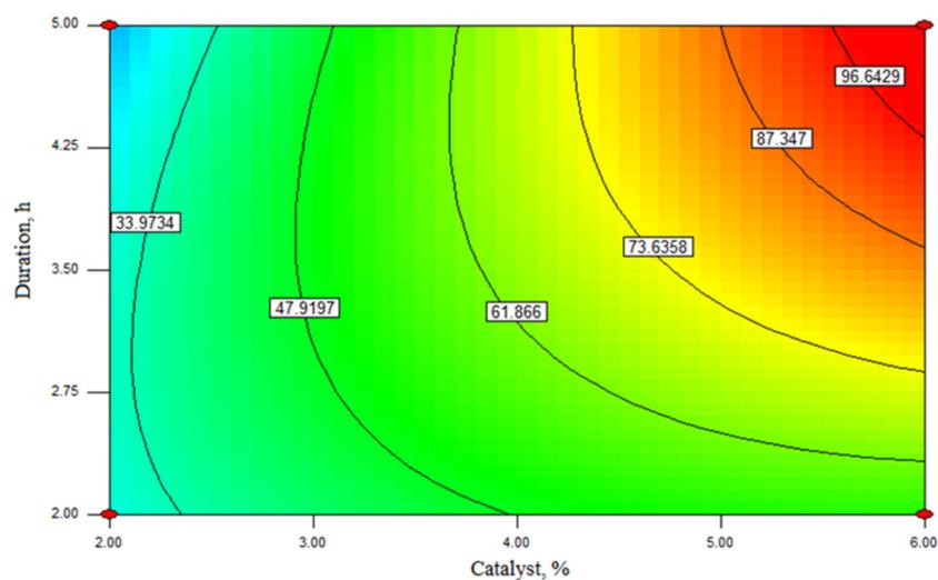
**Figure 5.** Response surface contour plot for the interaction between the duration and the catalyst amount for the ester yield when the process temperature is 64 °C and methanol-to-oil ratio is 12:1.
