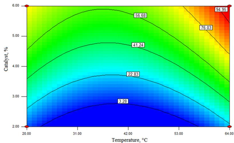
**Figure 7.** Response surface contour plot for the interaction between the catalyst amount and the temperature for the ester yield when the methanol-to-oil ratio is 12:1 and the process duration is 5 h.
