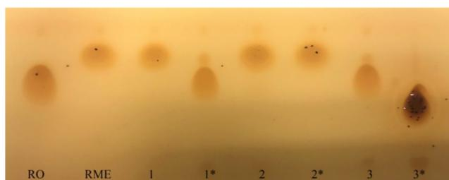
**Figure 2.** Reaction products of rapeseed oil transesterification with methanol using different fractions of dolomite: 1—0.63–0.315 mm, 1\*—0.63–0.315 mm, 2—0.315–0.1 mm, 2\*—0.315–0.1 mm, 3—0.1–0.063 mm, 3\*—0.1–0.063 mm, RO for rapeseed oil, RME for rapeseed oil methyl esters.
