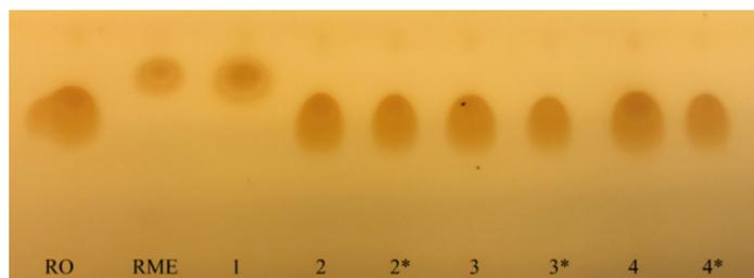
**Figure 1.** Reaction products of rapeseed oil transesterification with methanol using different natural catalysts: 1—dolomite, 2—glaucanitic sandstone, 2\*—glaucanitic sandstone, 3—opoka, 3\*—opoka, 4—serpentinite, 4\*—serpentinite, RO—rapeseed oil, RME—rapeseed oil methyl esters.
