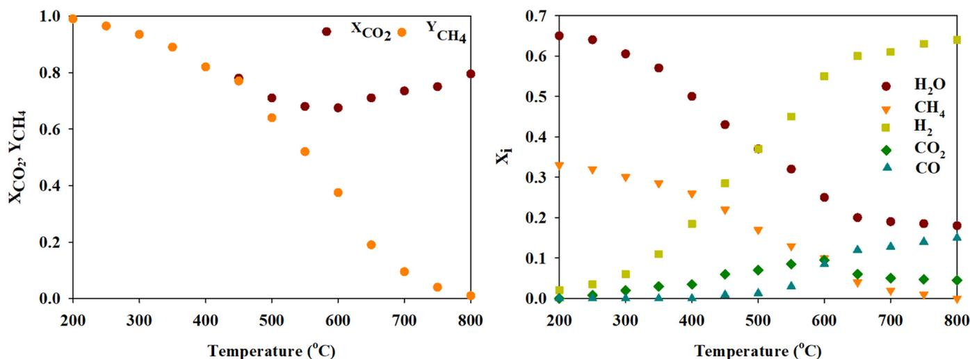
**Figure 6.** Equilibrium conversion rate (left) and the product fraction of CO<sub>2</sub> methanation at equilibrium (right),  $p = 1$  bar, H<sub>2</sub>/CO<sub>2</sub> = 4.
