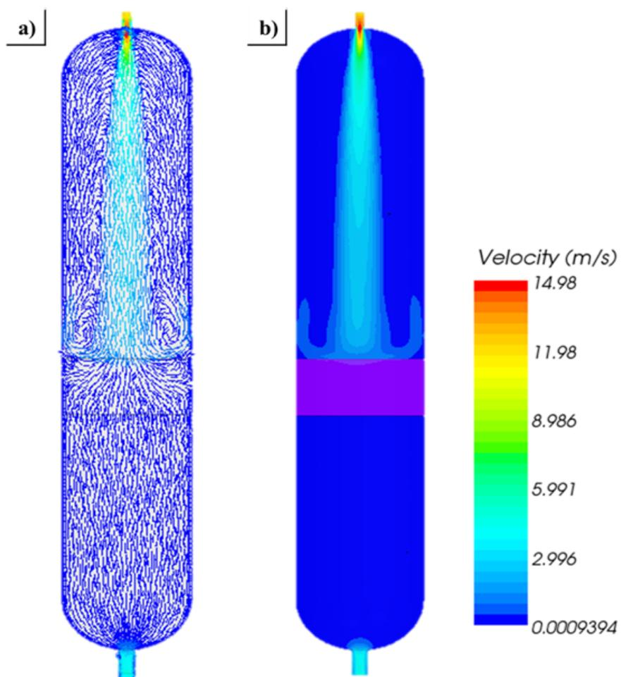
Figure 1. Velocity plot by cold-flow analysis: (a) velocity vector fields and (b) velocity magnitudes.
