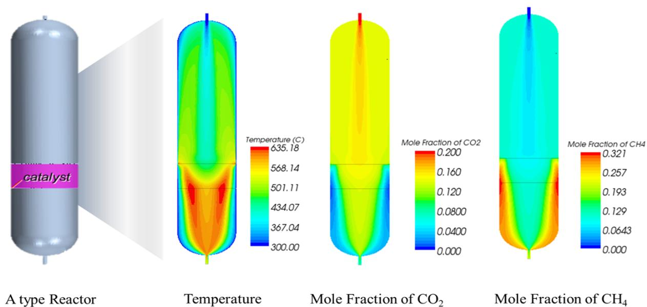
Figure 2. Reacting flow simulation for the A-type reactor.
