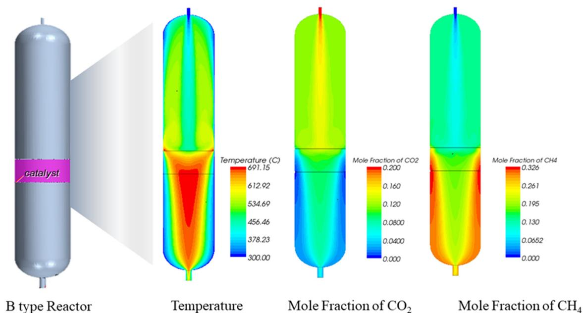
**Figure 3.** Reacting-flow simulation for the B-type reactor.
