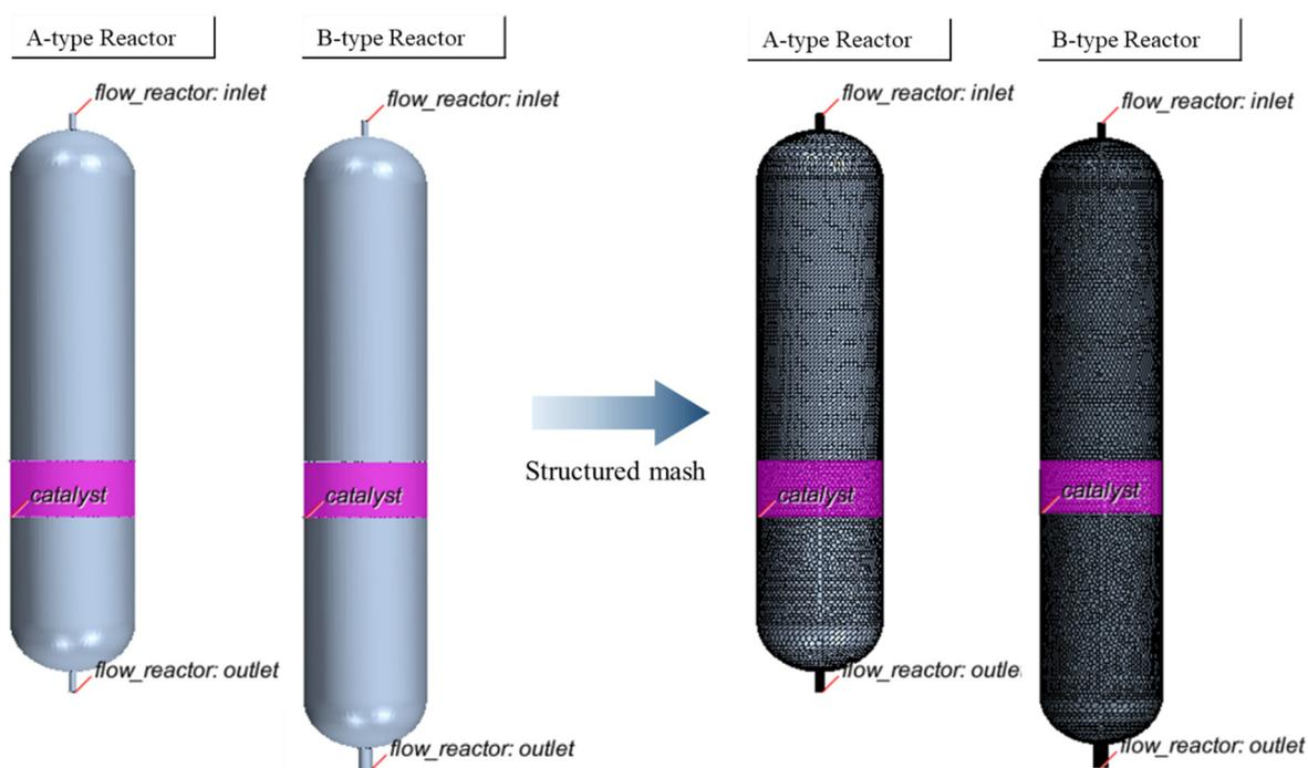
Figure 13. Computational domain and mesh generation of the two types of CO<sub>2</sub> methanation reactors.
