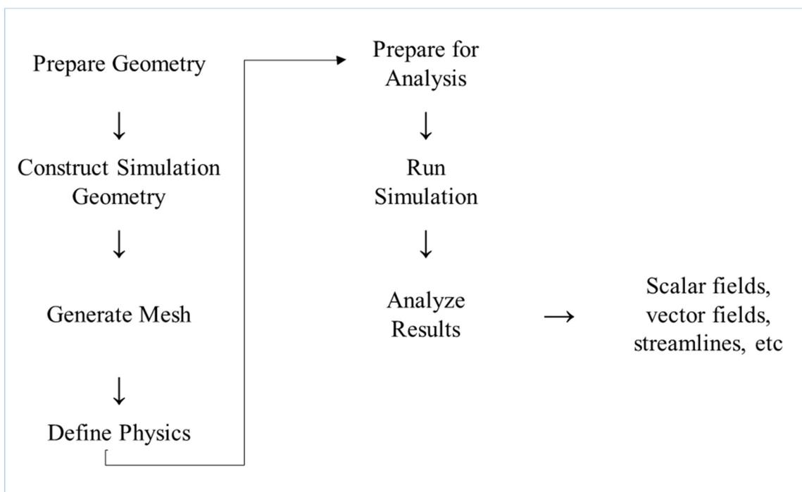
**Scheme 1.** Workflow process for simulation.
