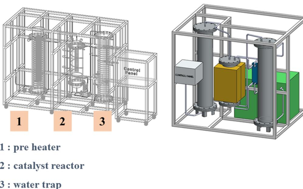
Figure 9. Pilot plant of CO<sub>2</sub> methanation in a sewage disposal plant in Korea.
