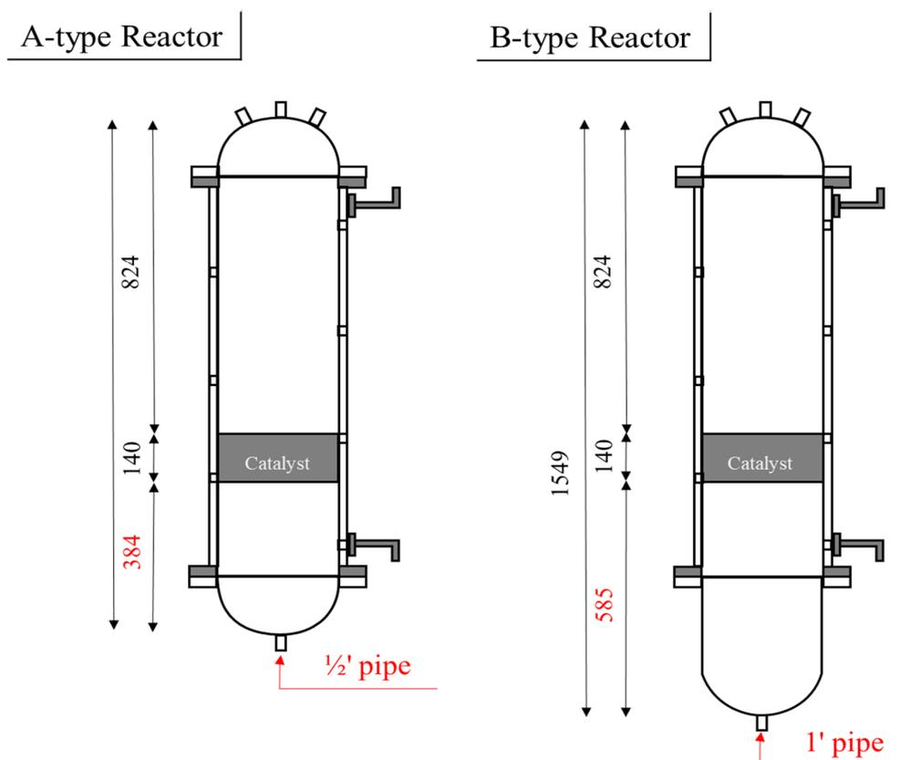
Figure 12. Schematic of the CO<sub>2</sub> methanation reactor.
