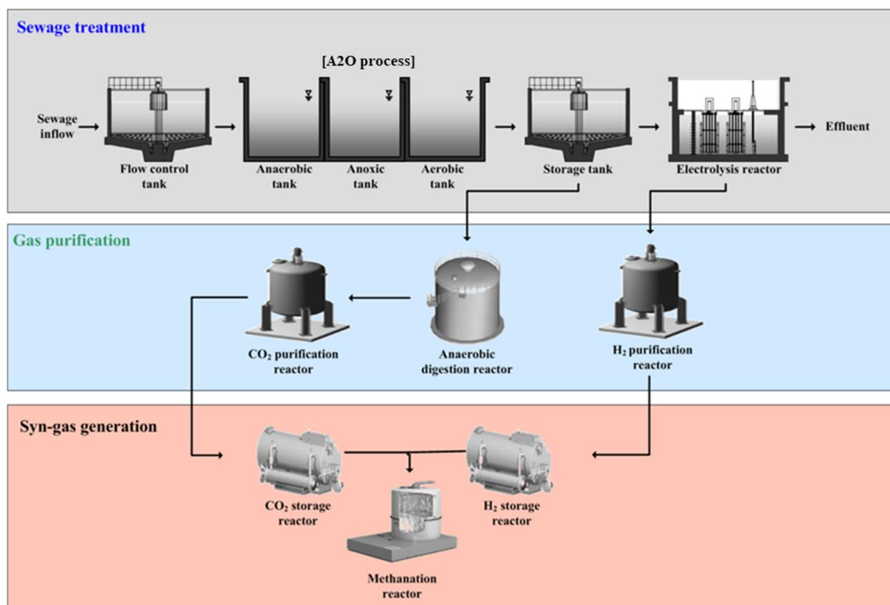
Figure 7. Process diagram of carbon resource integration.
