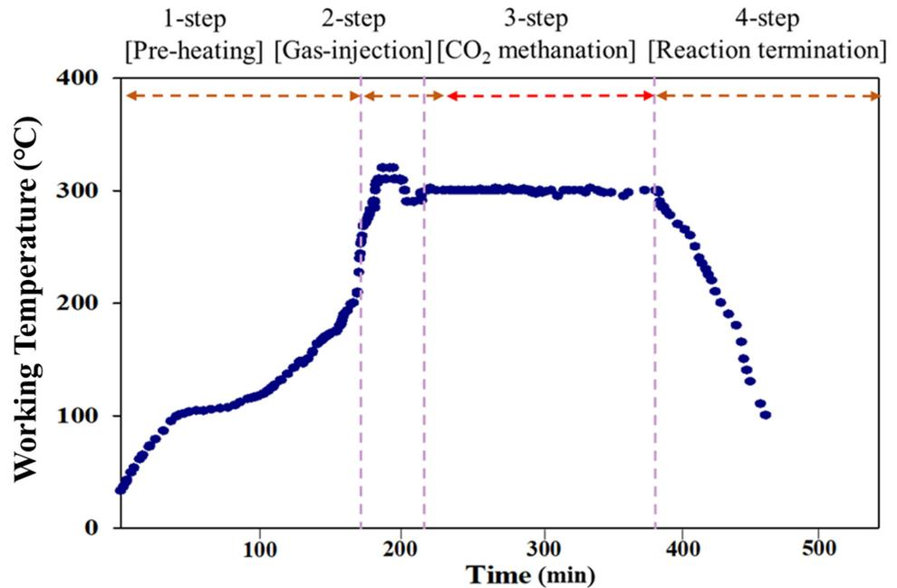
Figure 11. Four steps of the CO<sub>2</sub> methanation process.
