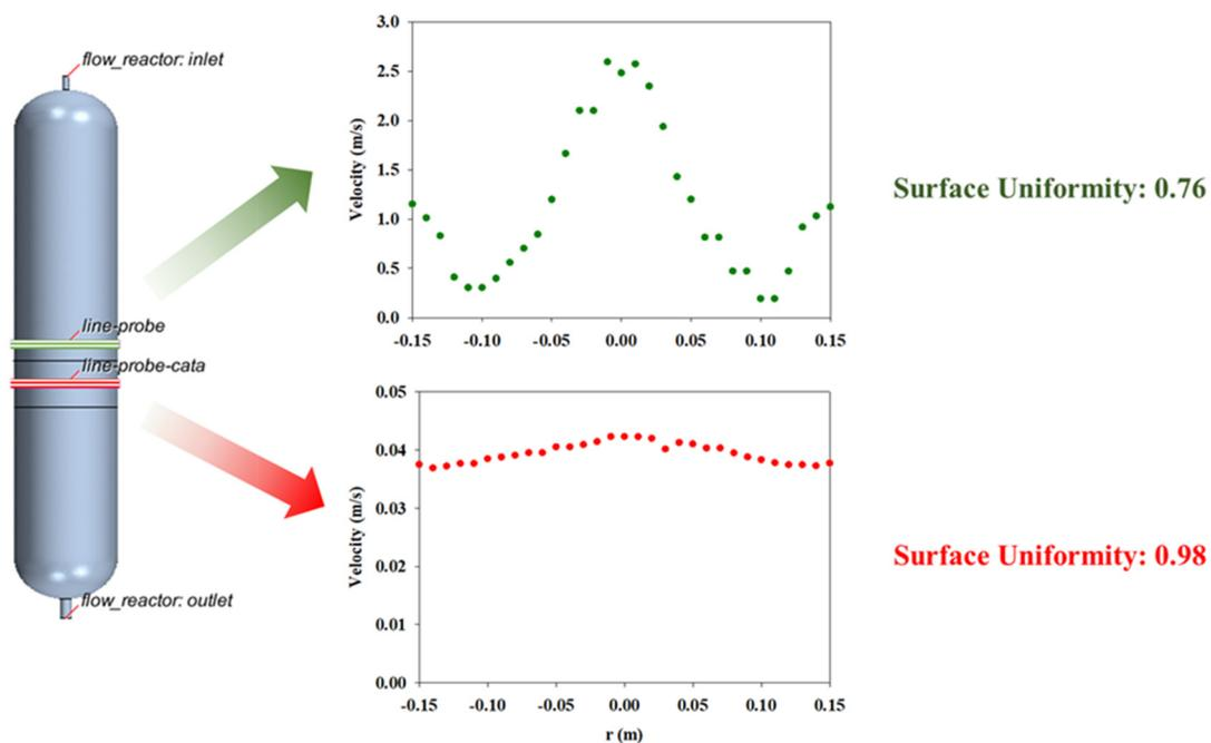
Figure 4. Hot-flow simulation result of the B-type reactor.
