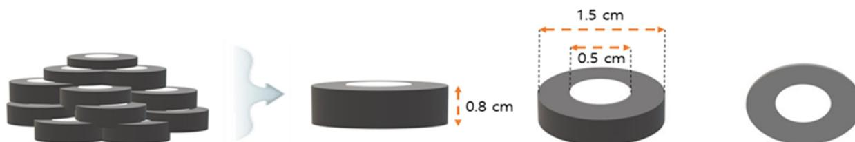
Figure 10. Structure of the manufactured pellet-type catalyst.
