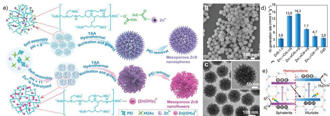
**Figure 16.** (a) Schematic illustration of the synthesis procedure of mesoporous ZnS nanostructures. (b,c) SEM and TEM images of mesoporous ZnS-1.0, respectively. (d) Photocatalytic HER of mesoporous  $Zn_xCd_{1-x}S$  with different Cd content. (e) Schematic view of a photocatalytic charge transfer mechanism for mesoporous  $Zn_{0.56}Cd_{0.44}$  in  $H_2$  evolution reaction. [149] Copyright 2021, Wiley-VCH.
