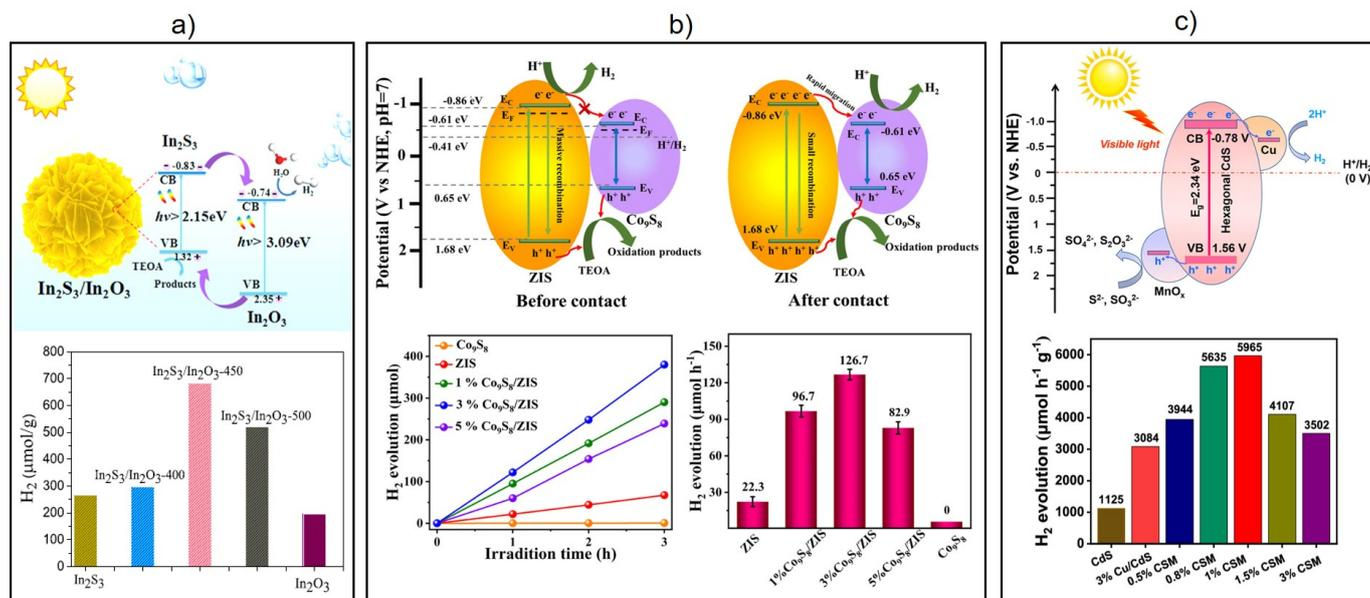
**Figure 10.** Schematic illustration of photocatalytic hydrogen evolution mechanism and corresponding HER plots for different metal sulfide and metal oxide heterostructures. (a)  $\text{In}_2\text{S}_3/\text{In}_2\text{O}_3$  [86] Copyright 2022, Elsevier. (b)  $\text{Co}_9\text{S}_8/\text{ZnIn}_2\text{S}_4$  [87] Copyright 2022, American Chemical Society. (c)  $\text{Cu/CdS/MnO}_x$  [88] Copyright 2021, American Chemical Society.
