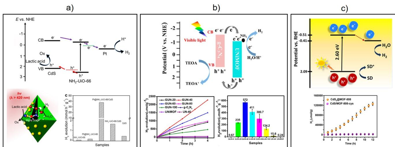
**Figure 13.** Proposed reaction mechanisms for the photocatalytic  $\text{H}_2$  evolution and obtained  $\text{H}_2$  production rates over different MS-based heterojunction photocatalysts. (a)  $\text{ZnIn}_2\text{S}_4@CoS_2$  [127] Copyright © 2022 Springer Nature. (b)  $\text{g-C}_3\text{N}_4/\text{UNiMOF}/\text{NiS}_2$  (GUN) [128] Copyright 2022, American Chemical Society. (c)  $\text{CdS@MOF-808}$  [129] Copyright © 2022, American Chemical Society.
