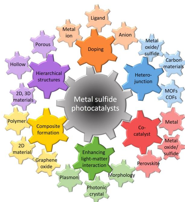
**Figure 4.** The most frequently employed strategies and representative components for enhancing hydrogen production over the metal sulfide photocatalysts. The figure was designed in accordance with the recent literature discussed in this review.
