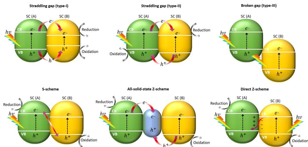
**Figure 6.** Schematic illustration of the most frequently reported charge transfer mechanisms for any photocatalytic systems. SC(A) and SC(B) stand for the two different semiconductor components of the corresponding photocatalyst.
