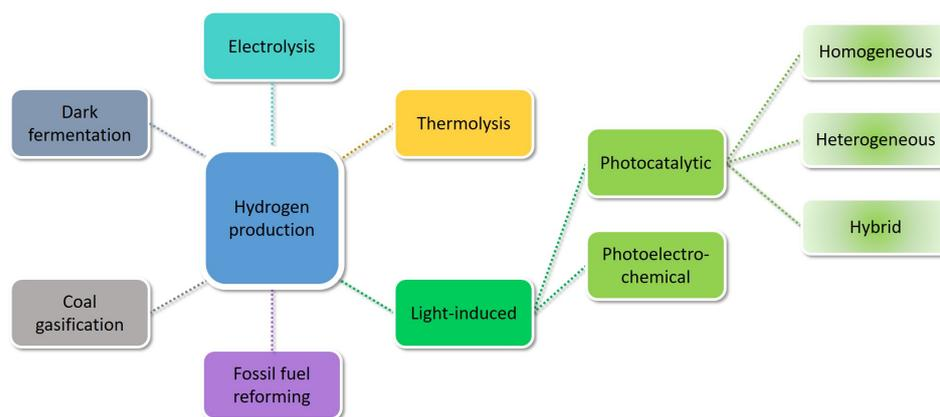
**Figure 1.** Most used possible routes for hydrogen generation. Currently, the solar-induced hydrogen evolution from water splitting is the most promising approach among others since it is environmentally benign, cost-effective, and offers the potential for high conversion efficiency.
