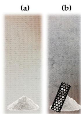
**Figure 7.** The image of photocatalysts: (a) TiO<sub>2</sub> photocatalytic film on glass fiber mesh, (b) TiO<sub>2</sub>/CNT photocatalytic film on glass fiber mesh.
