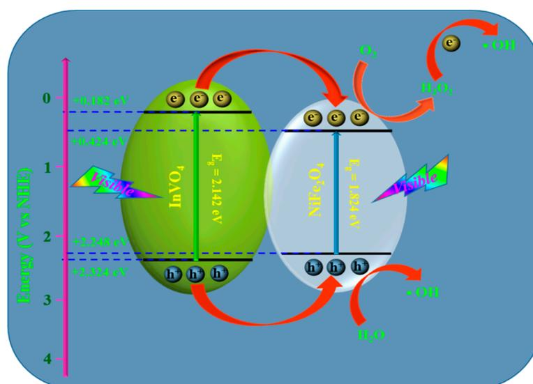
**Figure 12.** Photocatalytic degradation mechanism of TC molecules by the  $\text{InVO}_4/\text{NiFe}_2\text{O}_4$  nanocomposite under visible light.
