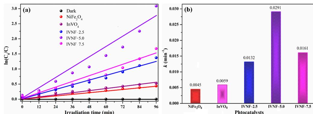
**Figure 9.** (a) Pseudo-first-order kinetics and (b) kinetic rate constants of the as-prepared catalysts.
