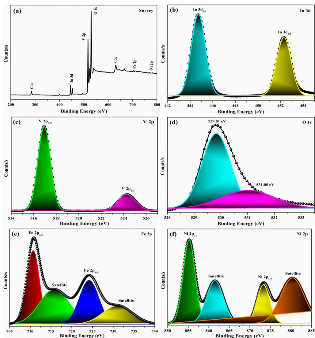
**Figure 5.** (a) Survey, (b) In 3d, (c) V 2p, (d) O 1s, (e) Fe 2p, and (f) Ni 2p high resolution X-ray photoelectron spectra of the IVNF-5.0 nanocomposite.
