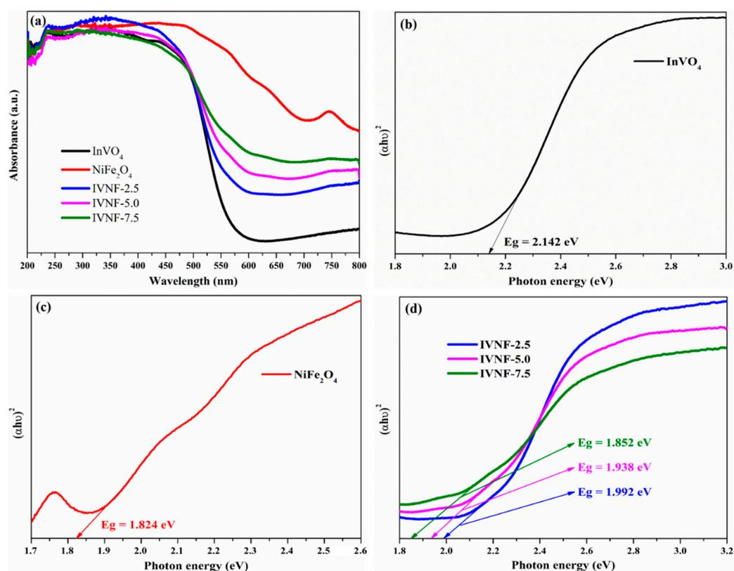
**Figure 6.** (a) Optical absorption spectra and (b–d) Tauc plots of the synthesized samples.
