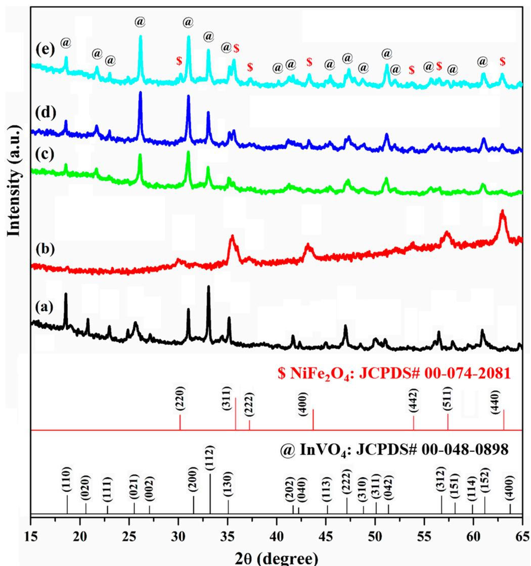
**Figure 1.** X-ray diffraction patterns of (a)  $\text{InVO}_4$ , (b)  $\text{NiFe}_2\text{O}_4$ , (c) IVNF-2.5, (d) IVNF-5.0, and (e) IVNF-7.5 nanocomposites.
