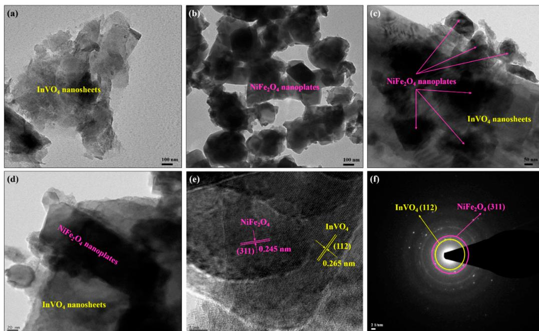
**Figure 3.** Transmission electron microscopy (TEM) images of (a)  $\text{InVO}_4$ , (b)  $\text{NiFe}_2\text{O}_4$ , and (c) IVNF-5.0; (d) high-resolution TEM image; (e) lattice fringes and (f) selected area electron diffraction patterns of the IVNF-5.0 nanocomposite.
