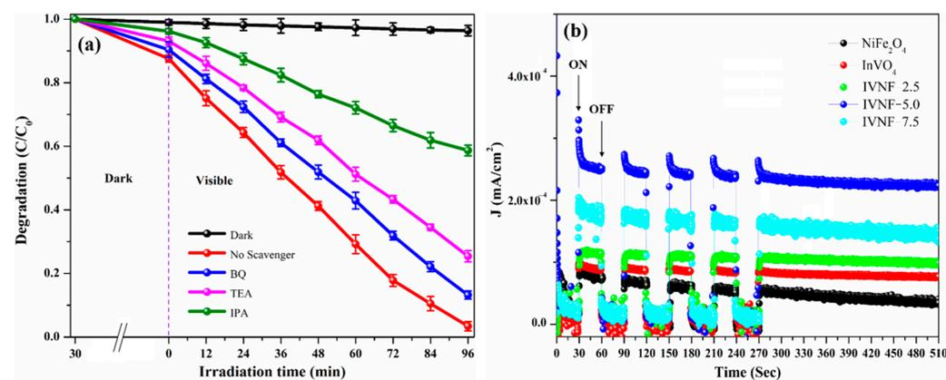
**Figure 11.** (a) Radical quenching experiment for the degradation of TC over IVNF-5.0 nanocomposite, and (b)  $I-t$  curves of the samples under the ON–OFF states.
