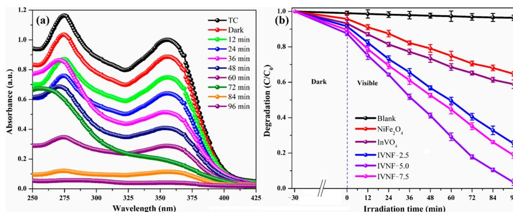
**Figure 8.** (a) Absorbance spectra for the degradation of tetracycline (TC) over the IVNF-5.0 nanocomposite and (b) degradation efficiency of the as-prepared samples.
