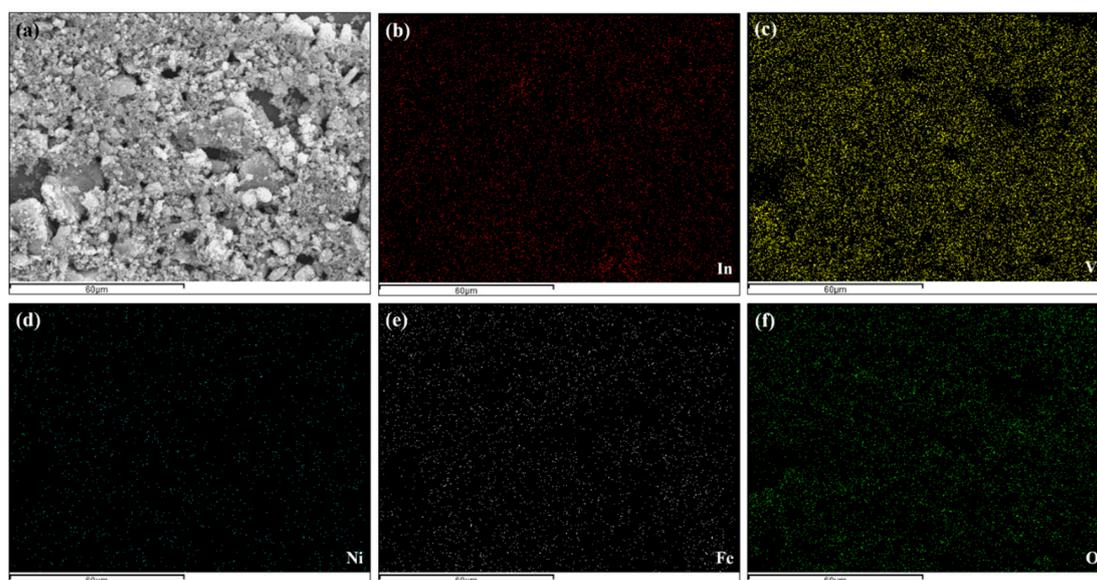
**Figure 4.** EDS elemental color mapping of the IVNF-5.0 nanocomposite. (a) Mapping region, (b) In, (c) V, (d) Ni, (e) Fe, and (f) O.
