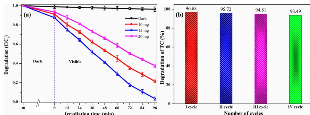
**Figure 10.** (a) Catalyst loading and (b) stability test over the IVNF-5.0 nanocomposite for the degradation of TC.
