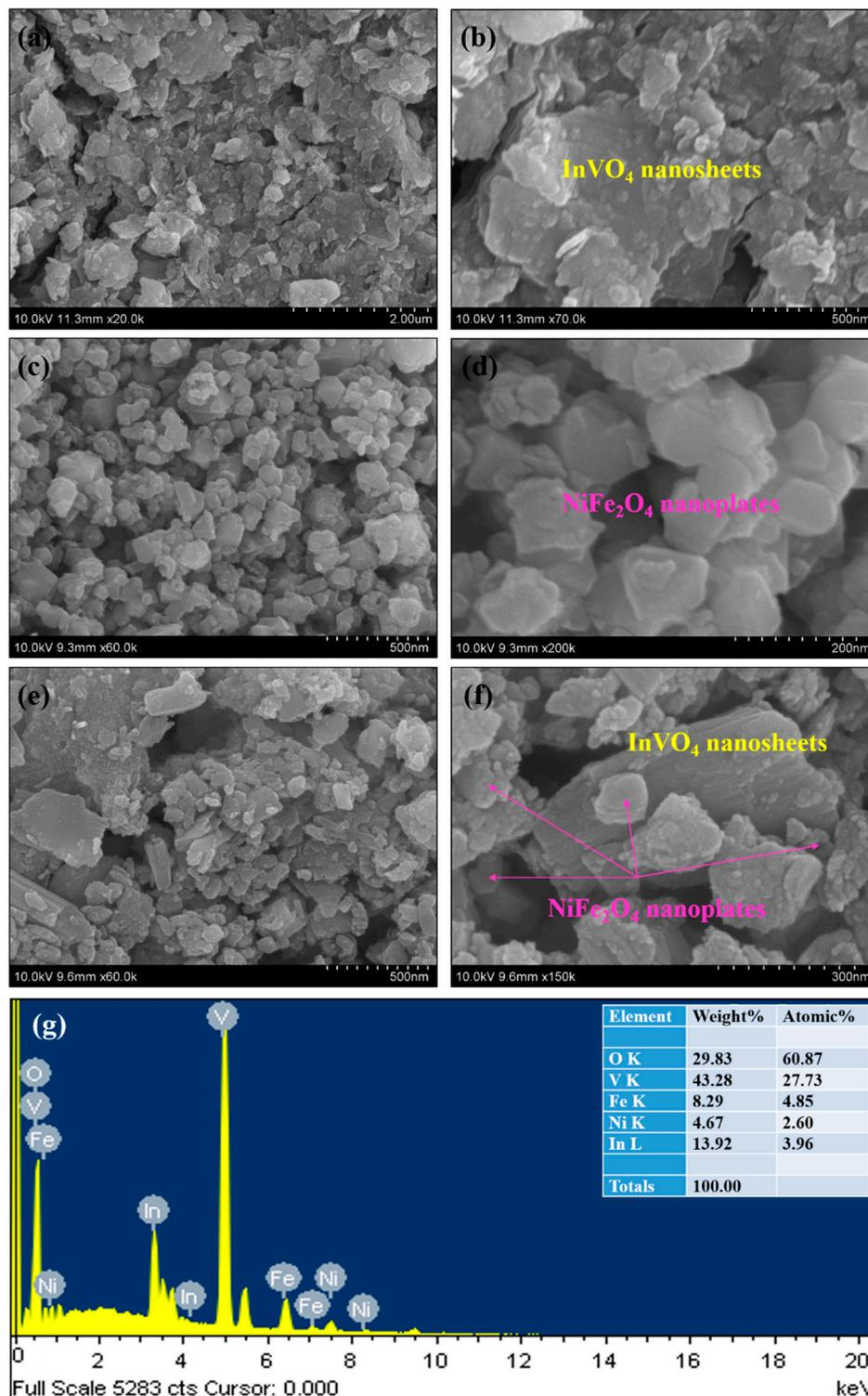
**Figure 2.** Scanning electron microscopy images of (a,b)  $\text{InVO}_4$  nanosheets, (c,d)  $\text{NiFe}_2\text{O}_4$  nanoplates, (e,f) IVNF-5.0 nanocomposite, and (g) energy-dispersive spectroscopy (EDS) analysis of the IVNF-5.0 nanocomposite.
