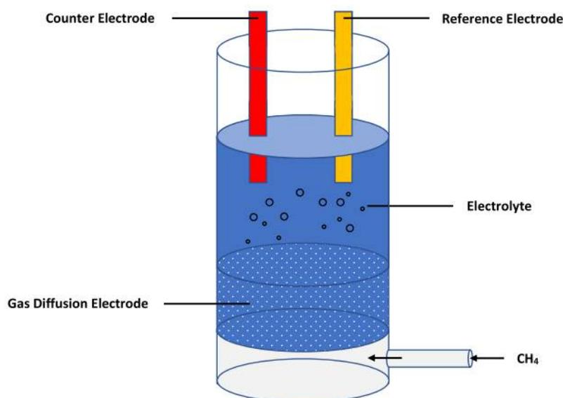
**Figure 1.** Scheme of the electrochemical reactor described by Rocha et al. [41].
