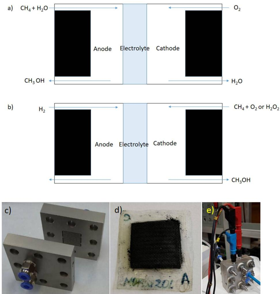
**Figure 2.** Fuel Cell Basic architecture: oxidation of methane (a) at the anode side and (b) at the cathode side. (c) reactor plates, (d) Membrane-electrode assemble, (e) reactor type fuel cell.
