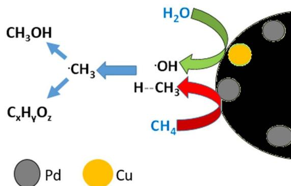
**Figure 4.** Partial methane oxidation with bifunctional PdCu/C electrocatalyst.
