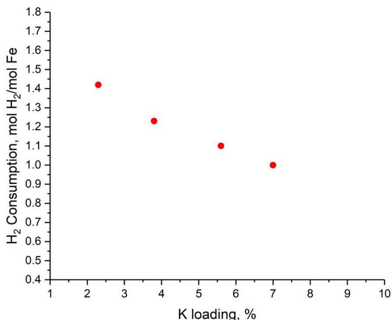
**Figure 4.** Total H<sub>2</sub> consumption during TPR for the fresh samples with different K loadings.
