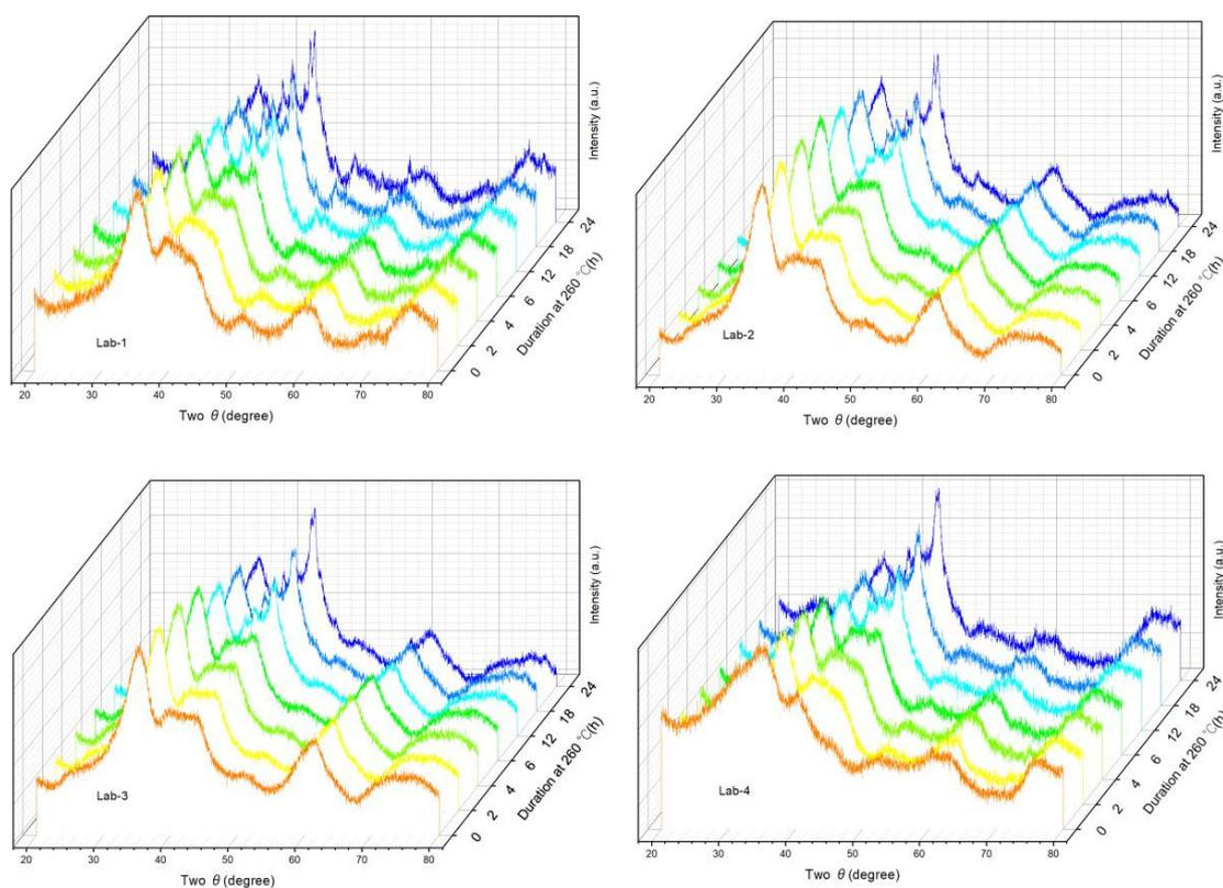
**Figure 6.** In situ XRD pattern of calcined samples during syngas reduction procedure ( $H_2/CO = 20$ , from an ambient temperature up to  $260\text{ }^\circ\text{C}$ , and maintained at  $260\text{ }^\circ\text{C}$ ).
