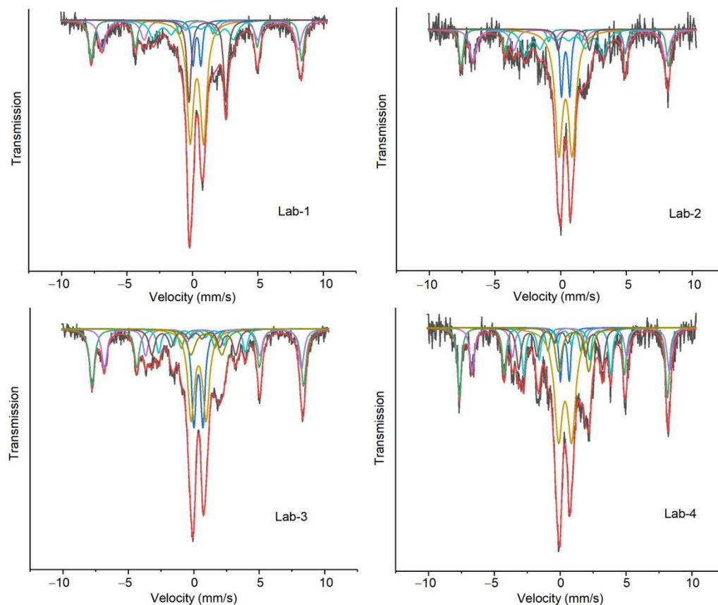
Figure 15. MES spectra of samples after FTS reaction.
