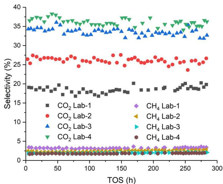
**Figure 11.** CO<sub>2</sub> and CH<sub>4</sub> selectivity with time on stream over the samples (reaction conditions: FBR, 2.3 MPa, 235 °C; Activation: H<sub>2</sub>/CO = 20, 260 °C, 24 h).
