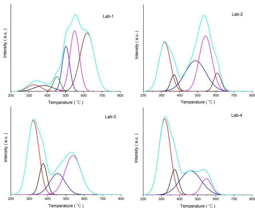
**Figure 7.** Peak splitting and fitting of H<sub>2</sub>-TPH profiles of the four catalyst samples (color correspondance by, red: carbidic carbon; black: amorphous carbon; green:  $\beta$  carbon; blue: bulk carbon 1; purple: bulk carbon 2; brown: bulk carbon 3).
