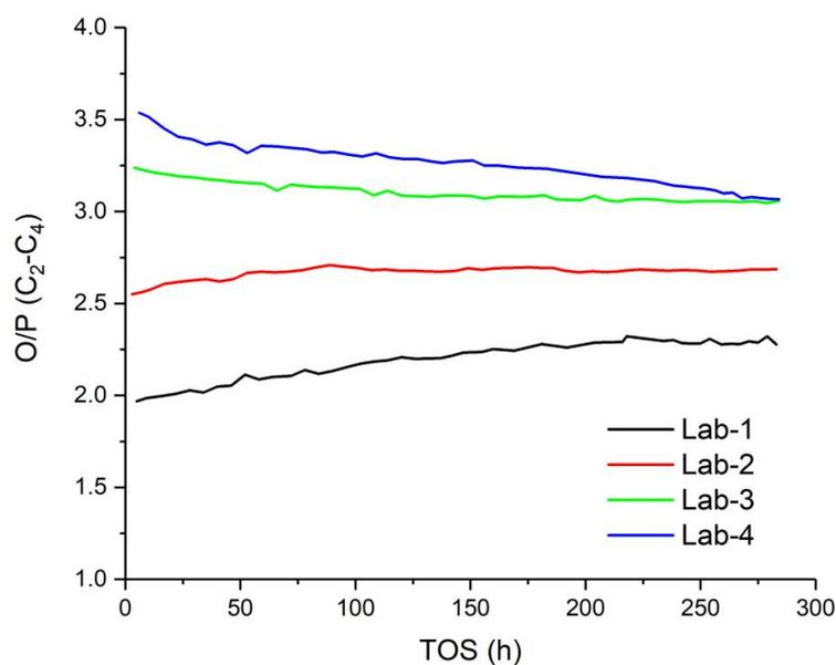
**Figure 12.** Olefin-to-paraffin ratio in the C<sub>2</sub>–C<sub>4</sub> section with time in-stream over the samples (reaction conditions: FBR, 2.3 MPa, 235 °C; Activation: H<sub>2</sub>/CO = 20, 260 °C, 24 h).
