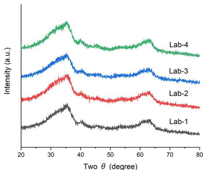
**Figure 1.** XRD pattern of the calcined precursor samples.
