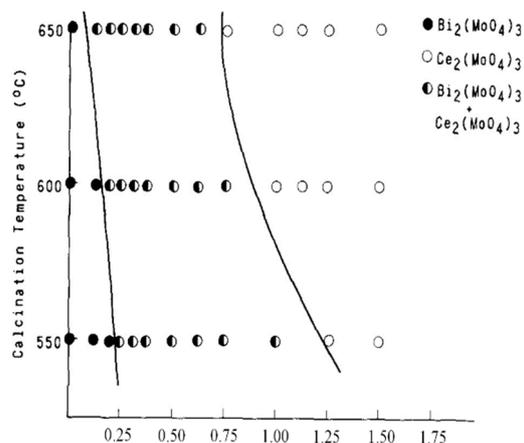
**Figure 5.** Partial phase diagram of  $\text{Bi}_{1-x}\text{Ce}_x\text{Mo}_3\text{O}_{12}$  where  $x$  is shown on the  $x$ -axis. Source with permission [34].
