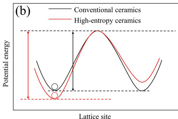
**Figure 7.** (a) Schematic diagram of lattice distortion effect in  $(\text{Ca}_{0.5}\text{Ce}_{0.5})(\text{Nb}_{0.25}\text{Ta}_{0.25}\text{Mo}_{0.25}\text{W}_{0.25})\text{O}_4$  high-entropy ceramics; (b) potential energy of ions in high-entropy and conventional ceramics. Source with permission: [168].
