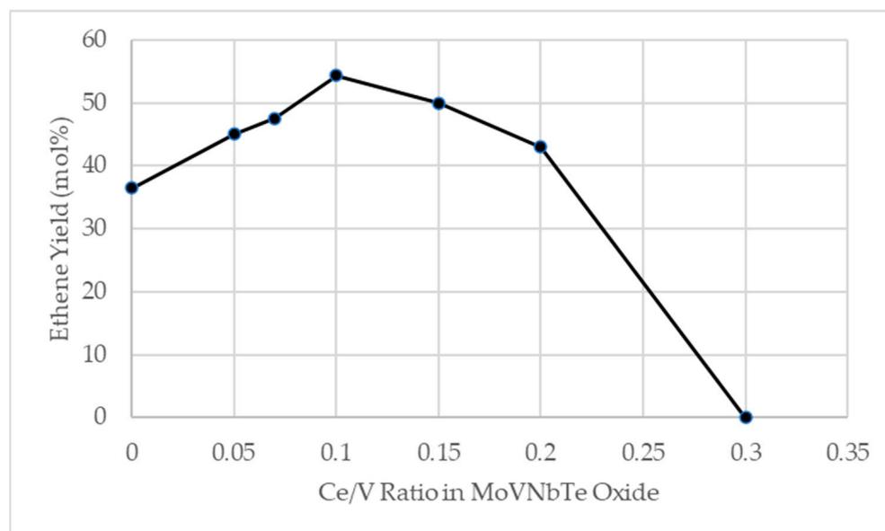
**Figure 4.** Ethane ODH with MoVTeNb Oxide catalyst with varying levels of cerium content. Source [69].
