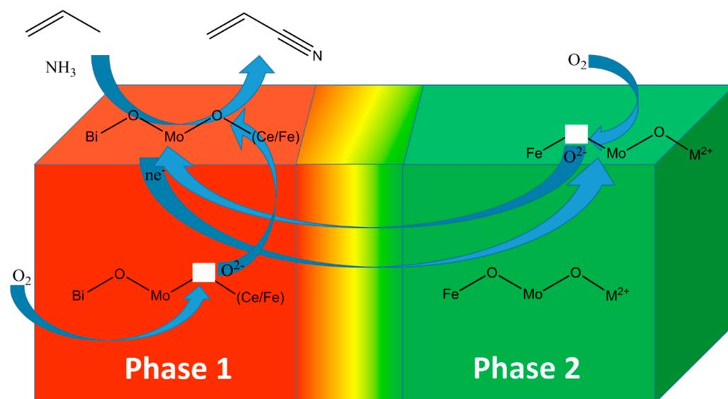
**Figure 2.** Schematic representation of multifunctionality in single and multiphase in an ammoxidation catalyst system [48].
