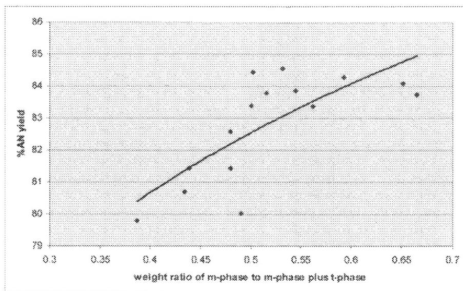
**Figure 3.** Rietveld X-ray diffraction analysis of cerium-containing mixed metal oxide acrylonitrile catalyst where m-phase ( $\text{Ce}_2(\text{MoO}_4)_3$ ) and t-phase refer to the monoclinic and tetragonal forms of the scheelite structure, respectively [49].
