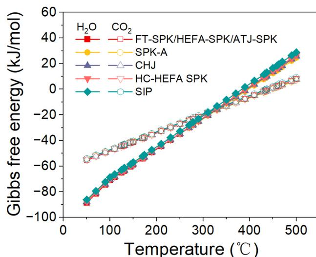
**Figure 1.** Comparison of  $\Delta G$  as a function of temperature for CO hydrogenation with H<sub>2</sub>O and CO<sub>2</sub> as products.
