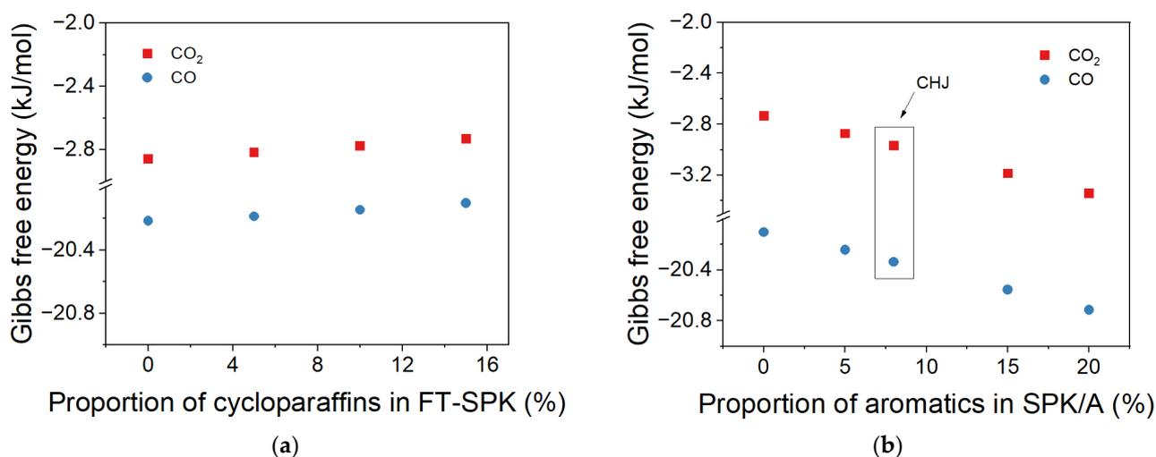
**Figure 7.** The effect of the proportion of cycloparaffins and aromatics in products on  $\Delta G$  ( $310^\circ\text{C}$ ). (a) Cycloparaffins in FT-SPK. (b) Aromatics in SPK/A.
