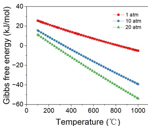
**Figure 6.** Effect of pressure and temperature on  $\Delta G$  for RWGS reaction.
