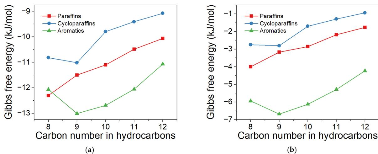
**Figure 5.** Effect of carbon number in products on  $\Delta G$  for CO<sub>2</sub> hydrogenation under different temperatures. (a) 270 °C. (b) 310 °C.
