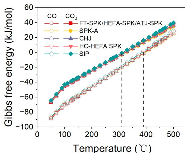
**Figure 2.** Temperature-dependent variation of  $\Delta G$  in the conversion pathway from CO/CO<sub>2</sub> to SAF.
