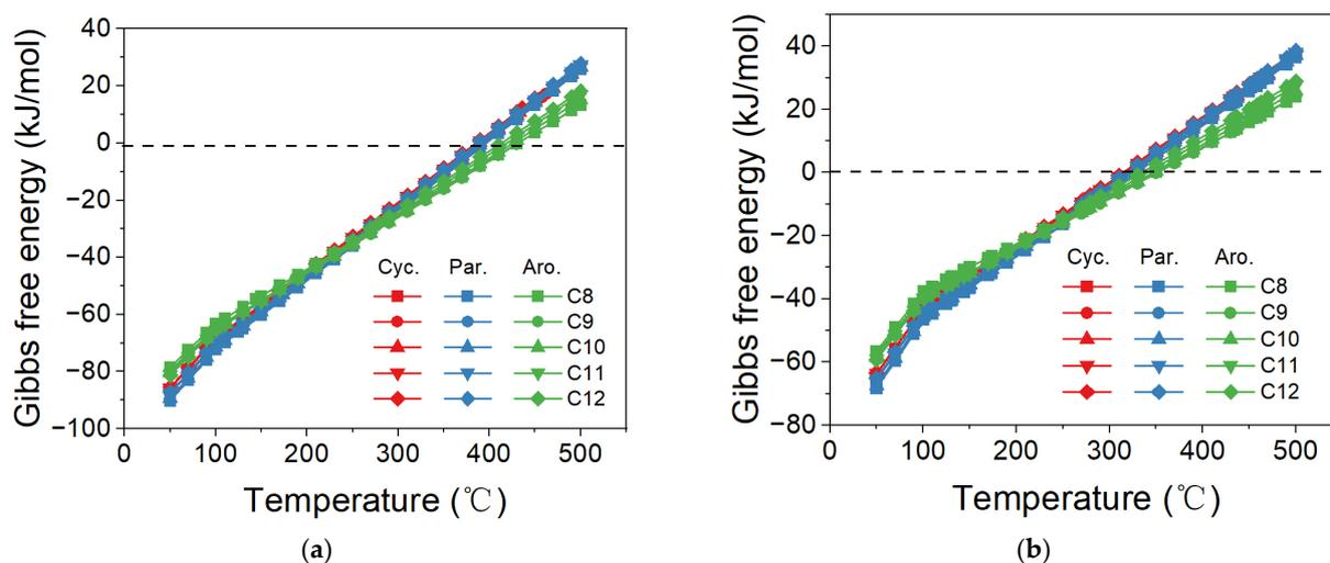
**Figure 3.** Temperature-dependent variation of  $\Delta G$  for the synthesis of different hydrocarbon components from CO/CO<sub>2</sub>. (a) CO. (b) CO<sub>2</sub>.
