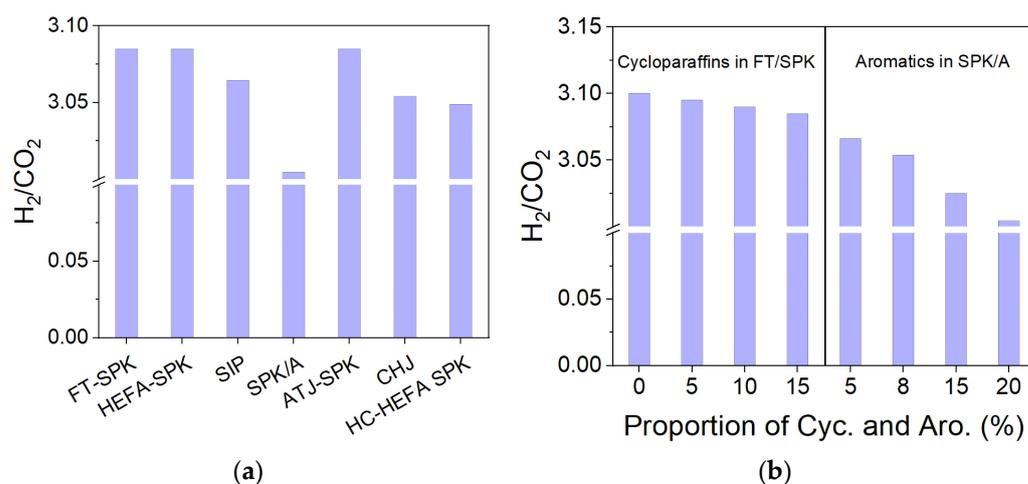
**Figure 8.** The effect of hydrocarbon types in the products on the H<sub>2</sub>/CO<sub>2</sub>. (a) Seven SAF products. (b) Products with different cycloparaffins and aromatics proportions.
