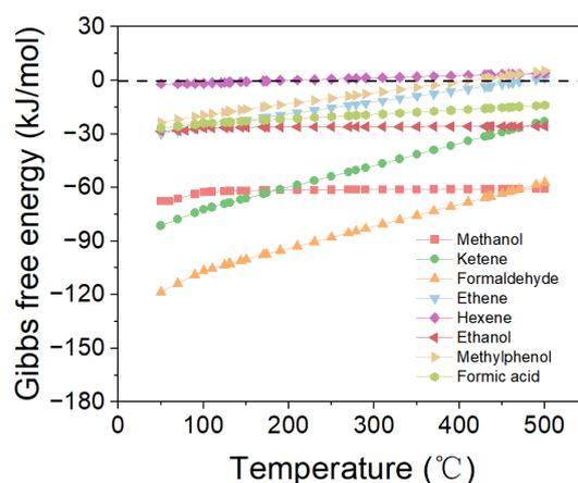
**Figure 10.** Temperature-dependent variation of  $\Delta G$  in the conversion pathway from specific intermediates to SAF.
