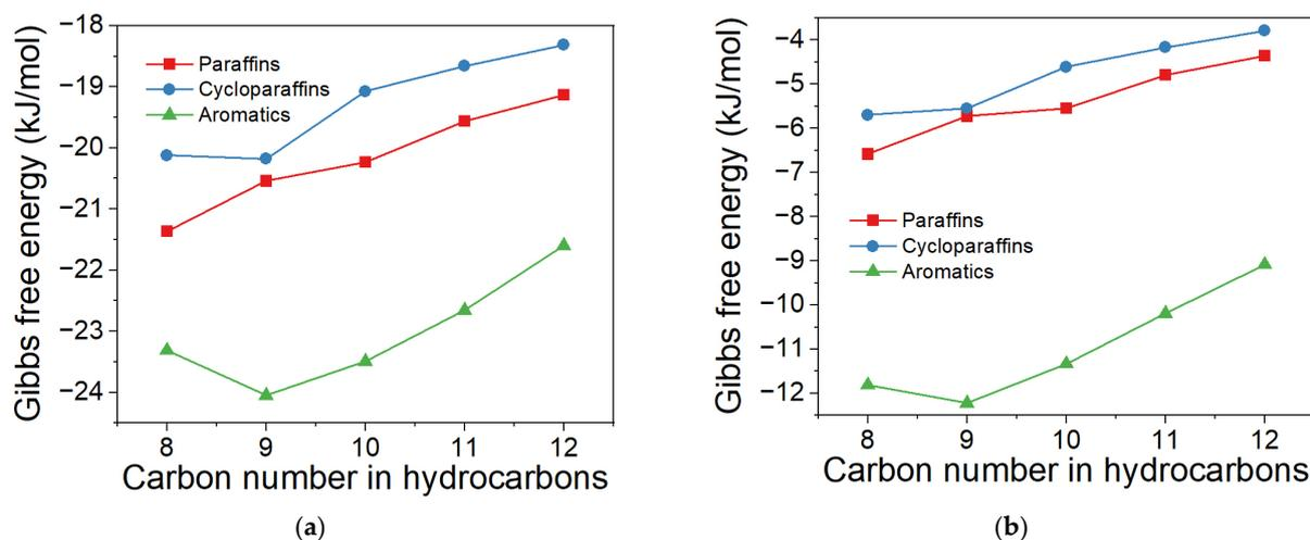
**Figure 4.** Effect of carbon number in products on  $\Delta G$  for CO hydrogenation under different temperatures. (a) 310 °C. (b) 370 °C.
