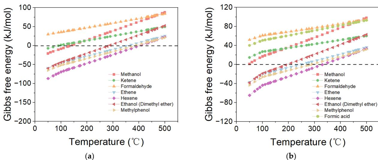
**Figure 9.** Temperature-dependent variation of  $\Delta G$  in the conversion pathway from CO/CO<sub>2</sub> to specific intermediates. (a) CO. (b) CO<sub>2</sub>.
