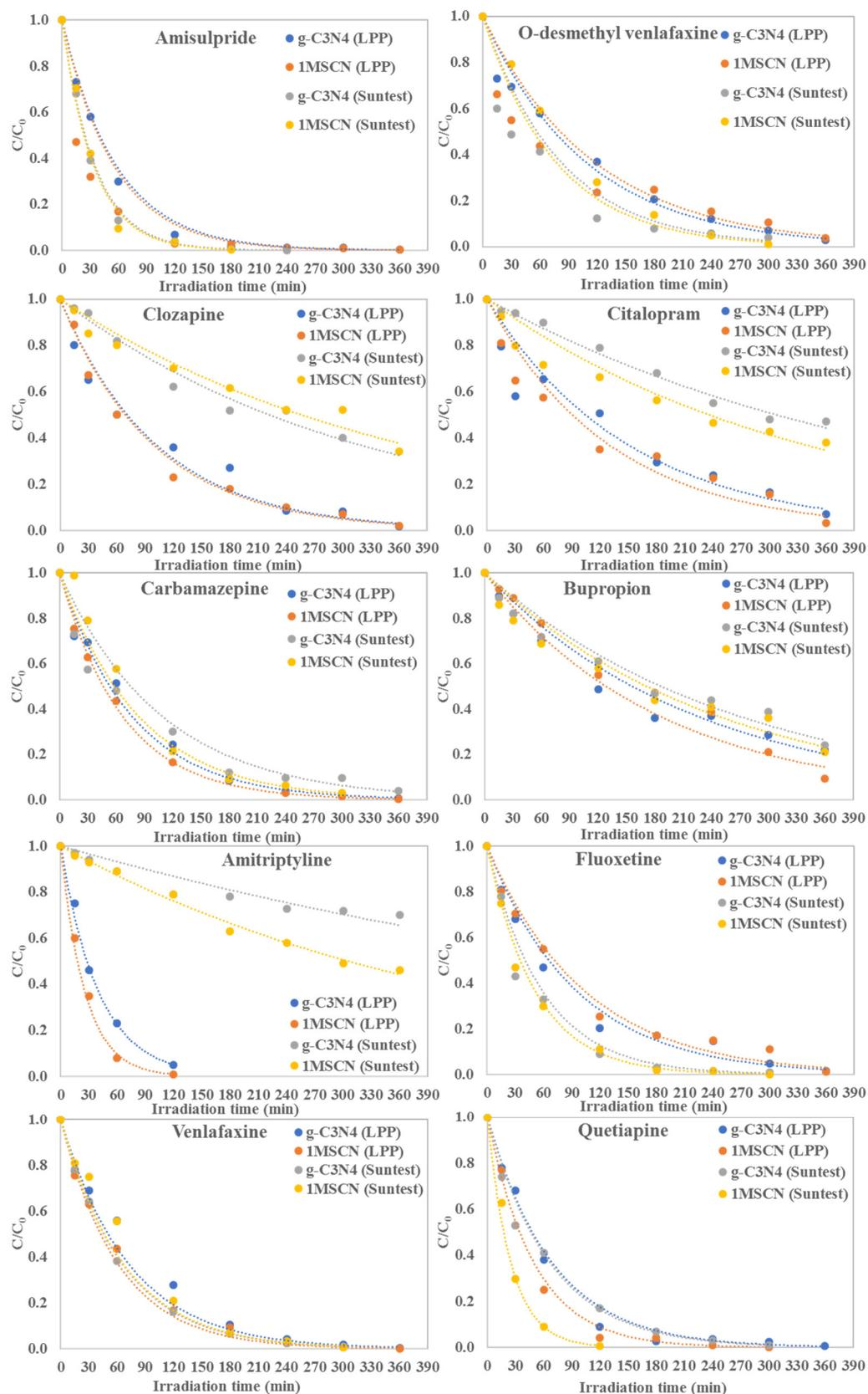
**Figure 1.** Photocatalytic degradation of psychiatric drugs using g-C<sub>3</sub>N<sub>4</sub> and 1MoS<sub>2</sub>/g-C<sub>3</sub>N<sub>4</sub> catalysts in lab-scale pilot plant (LPP) and in solar simulator (Suntest) as a function of irradiation time.
