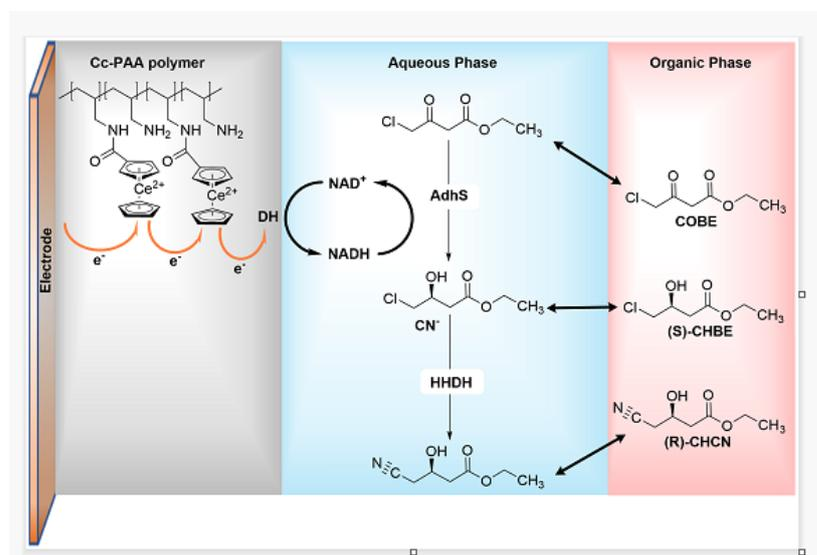
**Figure 13.** Preparation of (*R*)-CHCN through a biphasic bioelectrocatalytic approach.
