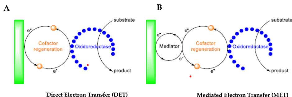
**Figure 15.** Direct (A) and mediated (B) interaction between oxidoreductase and electrode [29].
