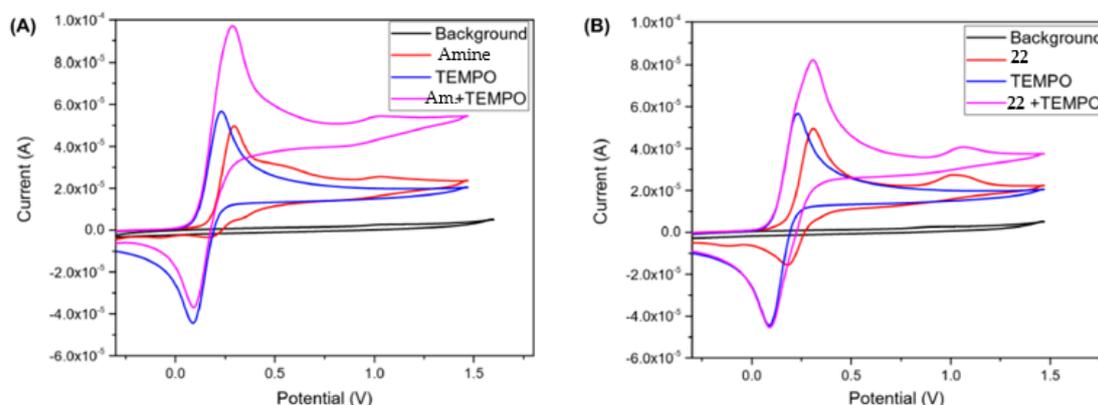
**Figure 8.** (A) Influence of TEMPO in the redox properties of the starting amine. (B) Influence of TEMPO in the redox properties of **22**.
