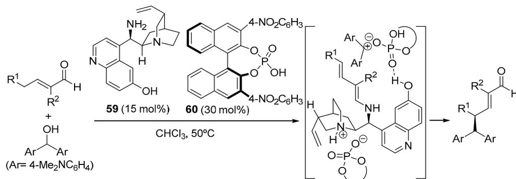
**Scheme 22.**  $\gamma$ -Alkylation of  $\alpha$ -substituted enals through  $S_N1$  reaction under cooperative primary amine Brønsted acid catalysis.
