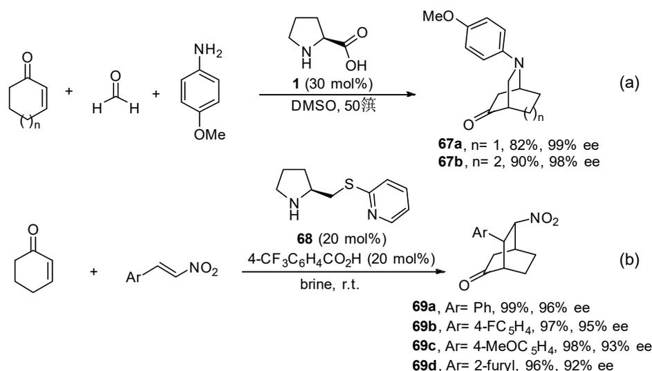
**Scheme 27.** Comparison between (a) proline and (b) pyridinium salt **68** in the nitroso-Diels–Alder reaction.
