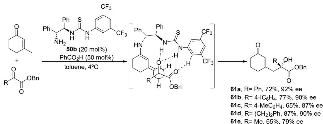
**Scheme 23.**  $\gamma$ -Functionalization of  $\beta$ -methylcyclohexenone through enantioselective aldol reaction.
