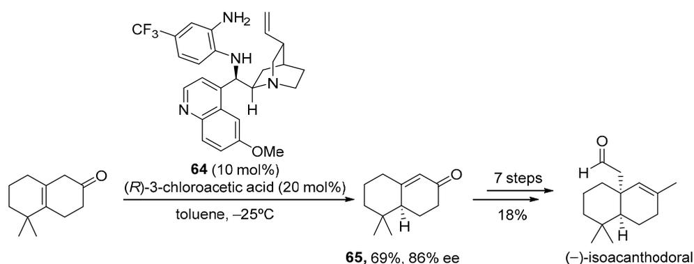
**Scheme 25.** Enantioselective isomerization of 3,4-disubstituted cyclohex-3-en-1-ones through protonation of dienamine intermediates and application to the total synthesis of (–)-isoacanthodoral.
