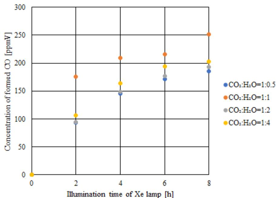
**Figure 10.** Concentration of the formed CO for double-layered Cu/TiO<sub>2</sub> and P<sub>4</sub>O<sub>10</sub>/TiO<sub>2</sub> with IR only illumination.
