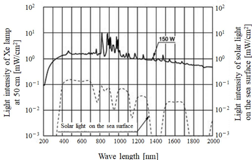
**Figure 16.** Light intensity spectrum data of the Xe lamp used in this study [36].
