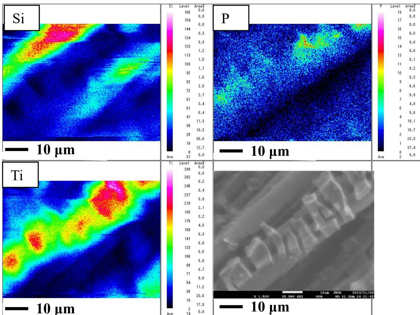
**Figure 2.** SEM and EPMA images of  $P_4O_{10}/TiO_2$  coated on the netlike glass disc, which was prepared in this study.
