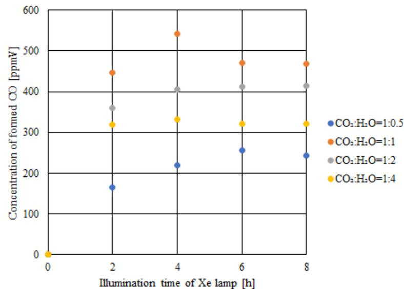
**Figure 6.** Concentration of the formed CO for double-layered Cu/TiO<sub>2</sub> and P<sub>4</sub>O<sub>10</sub>/TiO<sub>2</sub> with UV + VIS + IR illumination.
