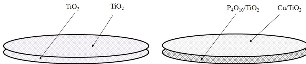
**Figure 5.** Schematic drawing of double-layered photocatalysts.
