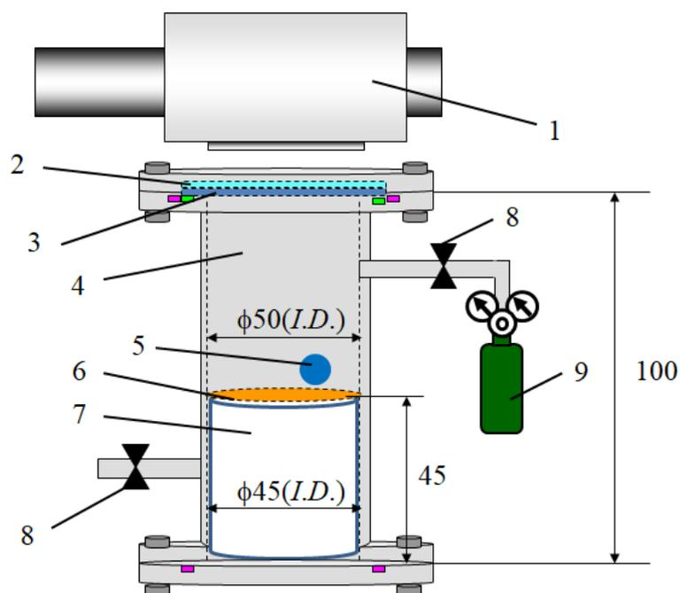
1. Xe lamp, 2. Sharp cut filter, 3. Quartz glass disc, 4. Stainless tube,
