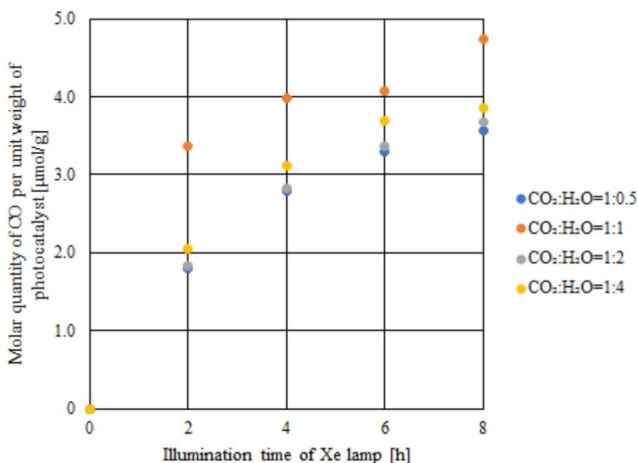
**Figure 11.** Molar quantity of CO per unit of the photocatalyst for double-layered Cu/TiO<sub>2</sub> and P<sub>4</sub>O<sub>10</sub>/TiO<sub>2</sub> with IR only illumination.
