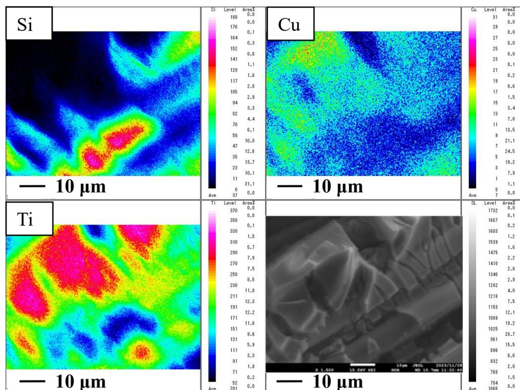
**Figure 1.** SEM and EPMA images of Cu/TiO<sub>2</sub> coated on the netlike glass disc, which was prepared in this study.
