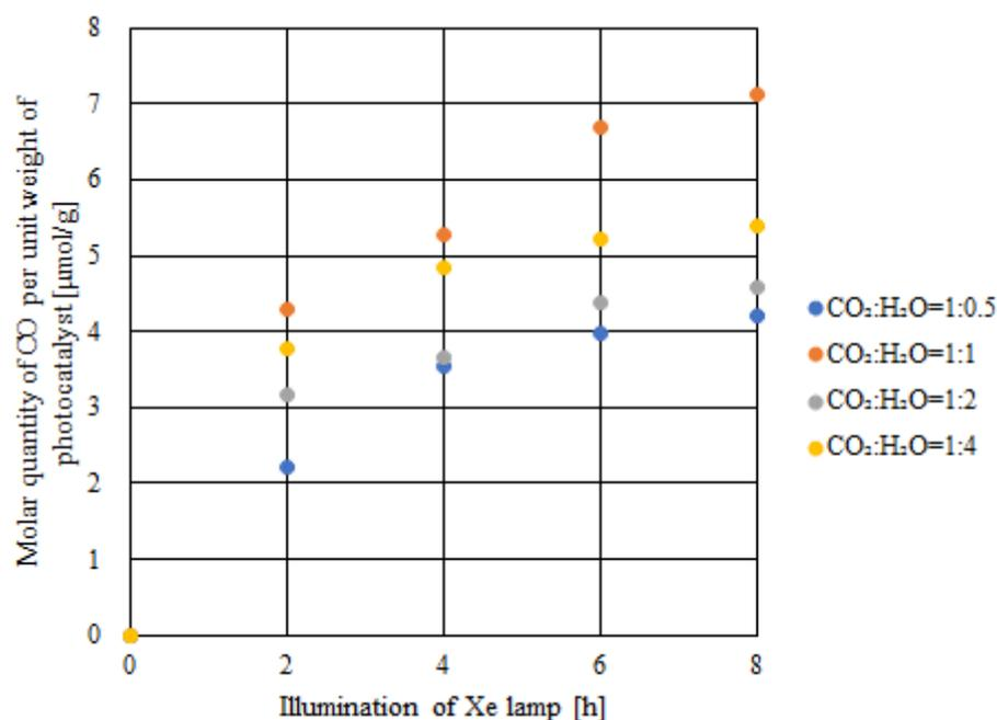
**Figure 9.** Molar quantity of CO per unit weight of the photocatalyst for double-layered Cu/TiO<sub>2</sub> and P<sub>4</sub>O<sub>10</sub>/TiO<sub>2</sub> with VIS + IR illumination.
