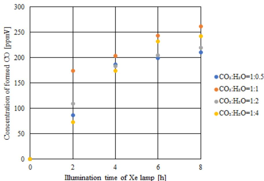
**Figure 3.** Concentration of the formed CO for double-layered TiO<sub>2</sub> with UV + VIS + IR illumination.
