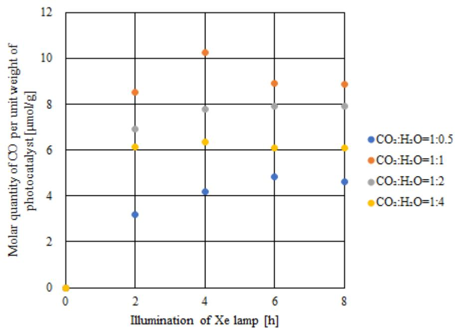
**Figure 7.** Molar quantity of CO per unit weight of the photocatalyst for double-layered Cu/TiO<sub>2</sub> and P<sub>4</sub>O<sub>10</sub>/TiO<sub>2</sub> with UV + VIS + IR illumination.
