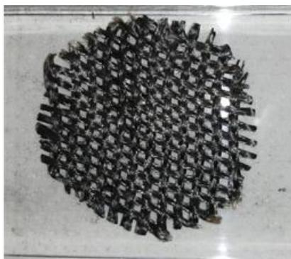
**Figure 12.** Photo of Cu/TiO<sub>2</sub> coated on the netlike glass disc.
