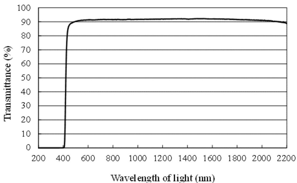
**Figure 15.** Light transmittance data of the sharp cut filter.
