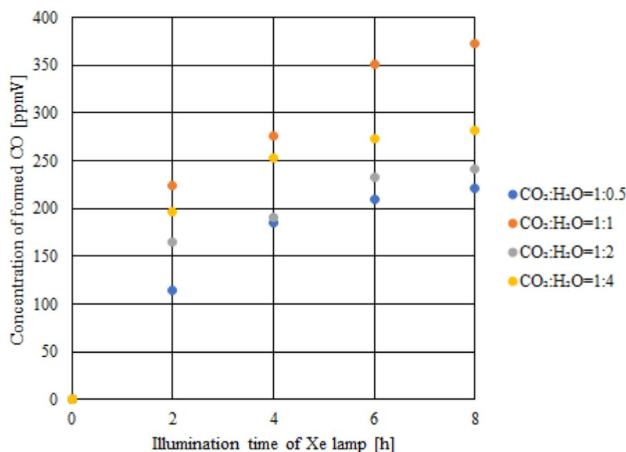
**Figure 8.** Concentration of the formed CO for double-layered  $\text{Cu}/\text{TiO}_2$  and  $\text{P}_4\text{O}_{10}/\text{TiO}_2$  with VIS + IR illumination.
