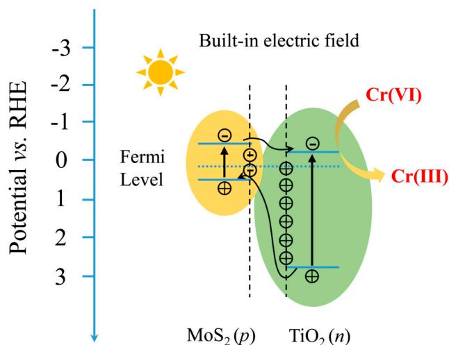
**Figure 10.** Schematic diagram for energy band of  $\text{MoS}_2/\text{TiO}_2$  NBs  $p-n$  heterojunction and photocatalytic reduction mechanism of Cr(VI).
