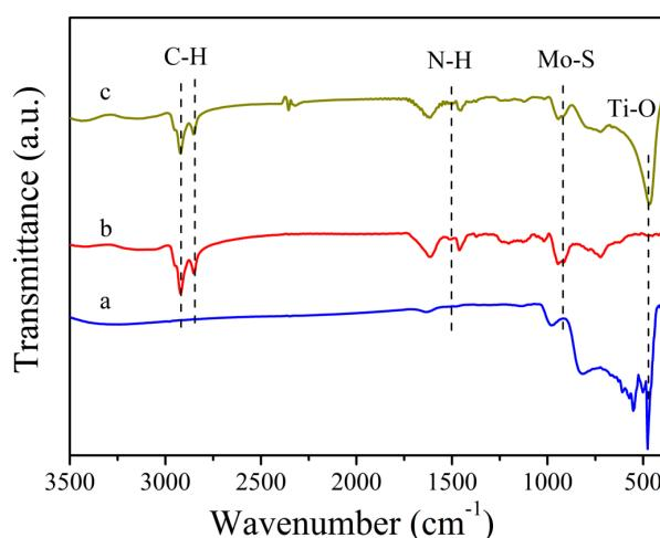
**Figure 5.** FTIR spectra of the as-prepared  $\text{TiO}_2$  NBs (a),  $\text{MoS}_2$  (b), and  $\text{MoS}_2/\text{TiO}_2$  NBs (c) heterojunction.
