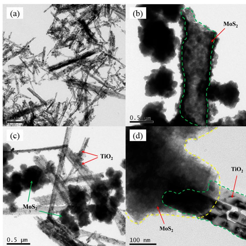
**Figure 3.** Transmission electron microscopy (TEM) images of: TiO<sub>2</sub> NBs (a); MoS<sub>2</sub> (b); and MoS<sub>2</sub>/TiO<sub>2</sub> NBs (c,d).
