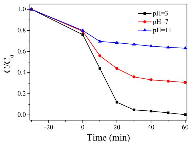
**Figure 8.** Degradation curves of Cr(VI) over  $\text{MoS}_2/\text{TiO}_2$  composite under different pH conditions.
