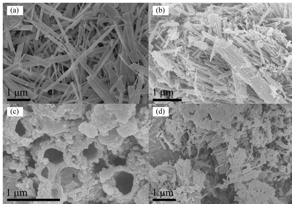
**Figure 2.** Scanning Electron Microscopy (SEM) images of: H<sub>2</sub>Ti<sub>3</sub>O<sub>7</sub> NBs (a); TiO<sub>2</sub> NBs (b); MoS<sub>2</sub> nanotubes (c); and MoS<sub>2</sub>/TiO<sub>2</sub> NBs heterojunctions (d).
