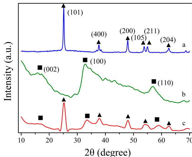
**Figure 1.** XRD patterns of:  $\text{TiO}_2$  nanobelts (NBs) (a);  $\text{MoS}_2$  nanotubes (NTs) (b); and  $\text{MoS}_2/\text{TiO}_2$  heterojunction (c).  $\blacktriangle$ , denotes the diffraction peak of  $\text{TiO}_2$  NBs;  $\blacksquare$ , the diffraction peak of  $\text{MoS}_2$  NTs.
