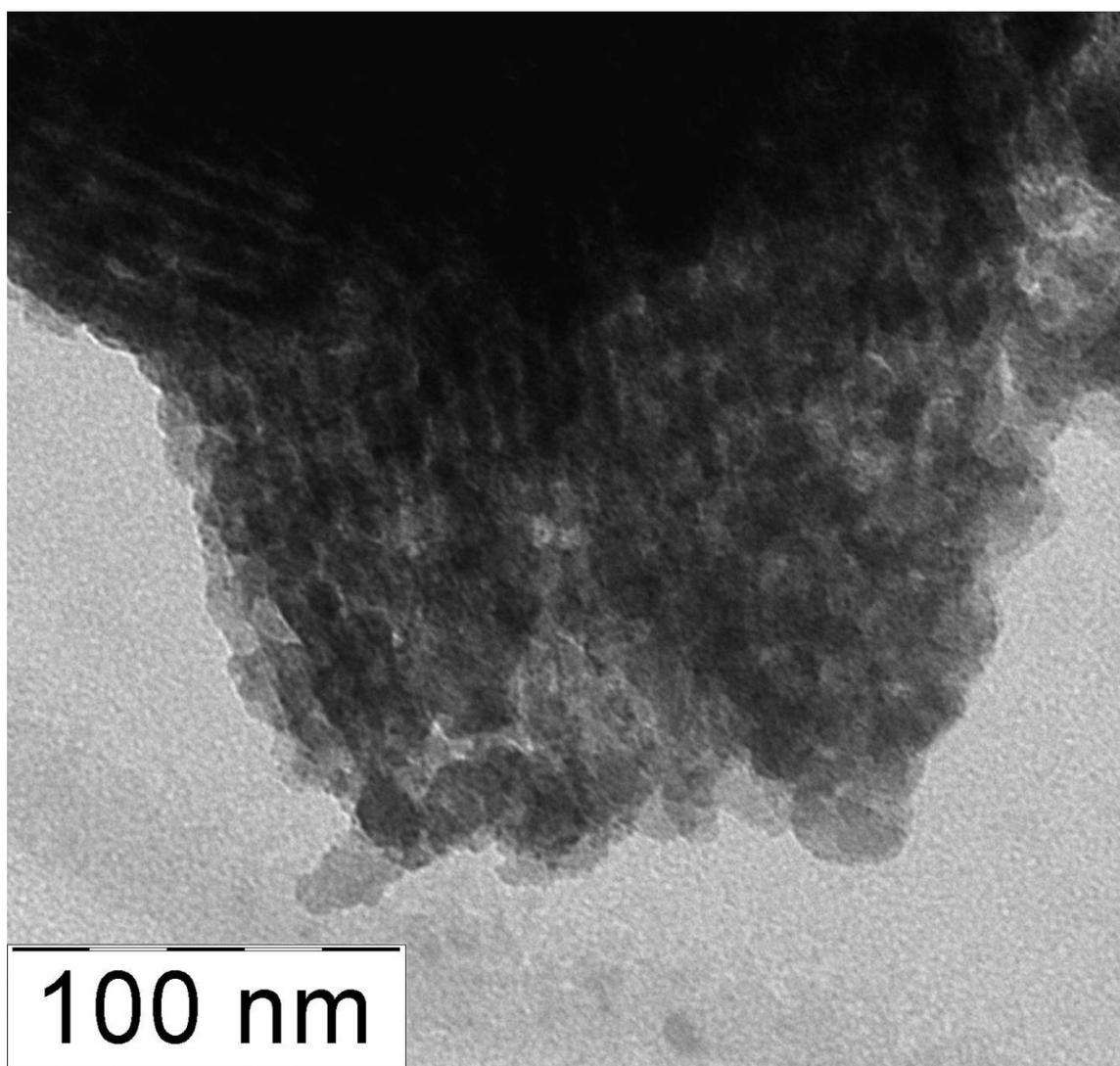
**Figure S3.** Maintenance of mesoporous structure in G2-dendr-*meso*-SiO<sub>2</sub>-Ru after reduction by aqueous NaBH<sub>4</sub>.
