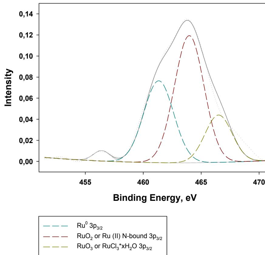
Figure S6. XPS spectrum G3-dendr-SiO<sub>2</sub>-Ru, Ru 3p line.
