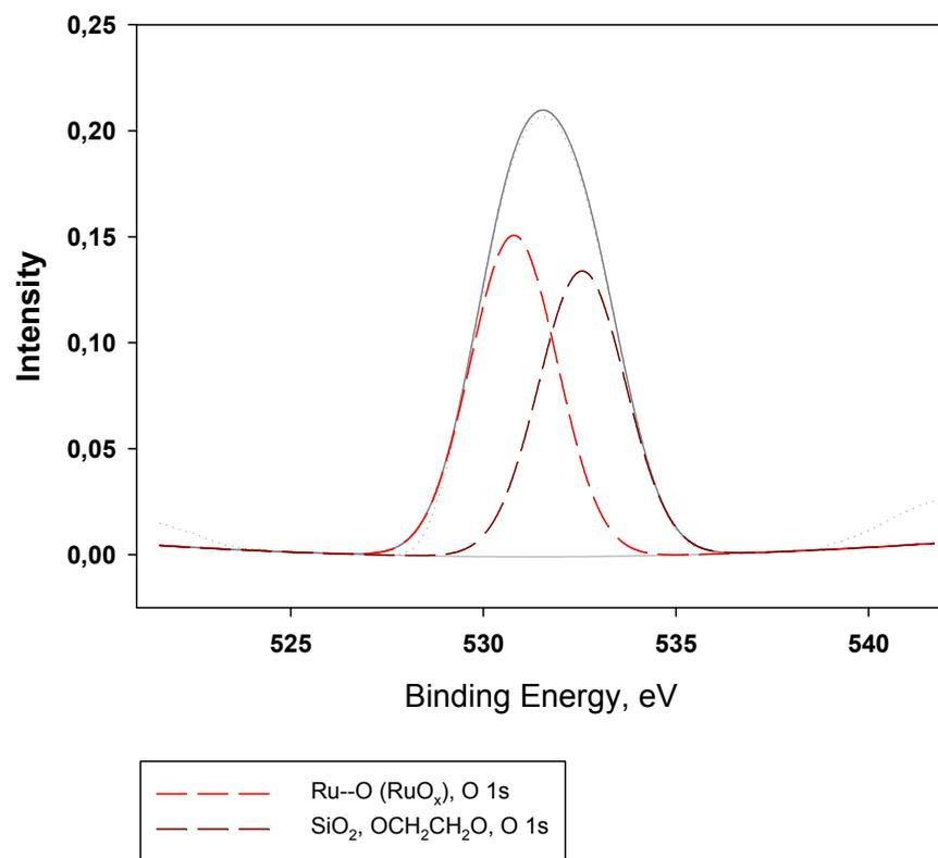
Figure S7. XPS spectrum of G2-dendr-*meso*-SiO<sub>2</sub>-Ru, O 1s line.
