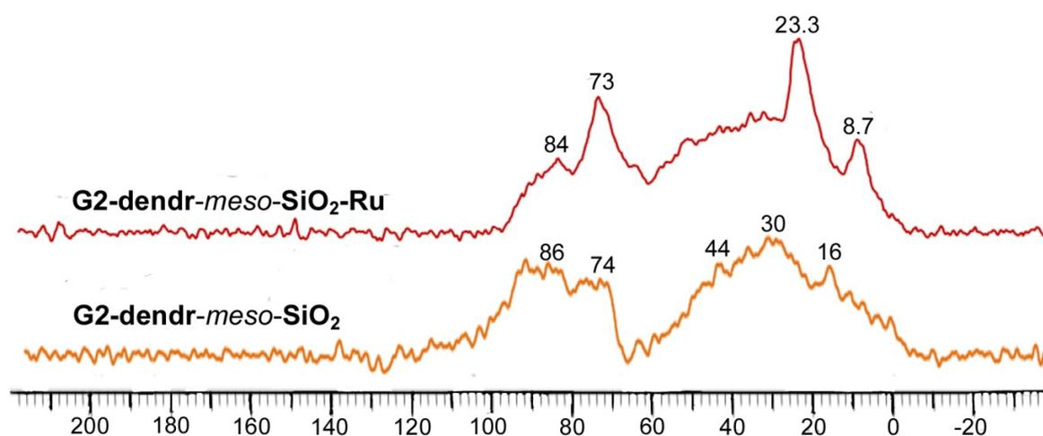
**Figure S1.** <sup>13</sup>C MAS NMR spectra of G2-dendr-*meso*-SiO<sub>2</sub>-Ru catalyst and its carrier.
