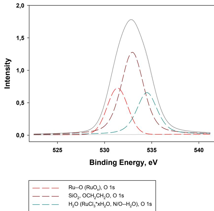
Figure S8. XPS spectrum G3-dendr-SiO<sub>2</sub>-Ru, O 1s line.
