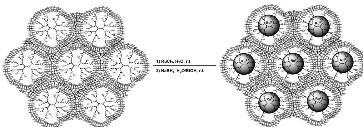
**Scheme S1.** Encapsulation of Ru nanoparticles into PPI dendrimers, immobilized in silica pores.
