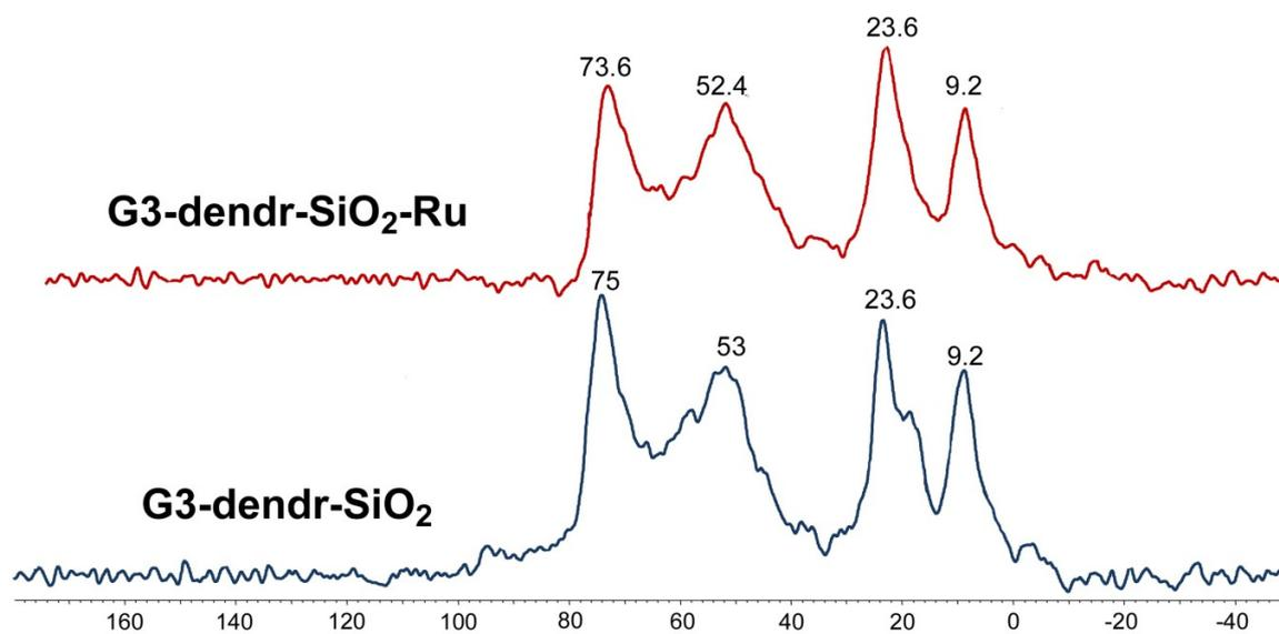
**Figure S2.**  $^{13}\text{C}$  MAS NMR spectra of G3-dendr-SiO<sub>2</sub>-Ru catalyst and its carrier.
