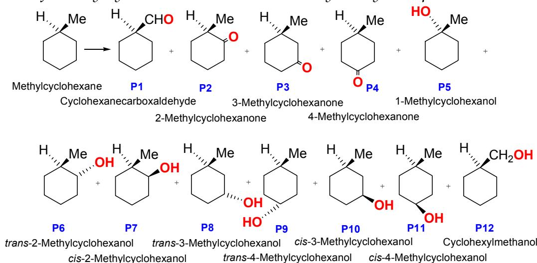
**Figure S1.** Isomeric products formed in the methylcyclohexane oxidation.
