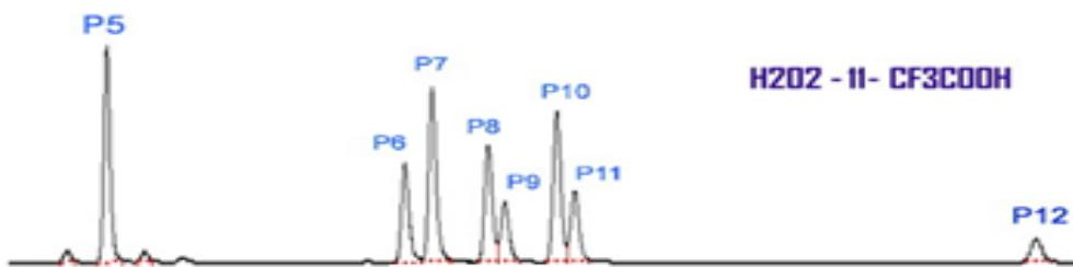
**Figure S2.** A chromatogram of products obtained in oxidations of methylcyclohexane by the “ $\text{H}_2\text{O}_2\text{-II-}\text{CF}_3\text{COOH}$ ” system.
