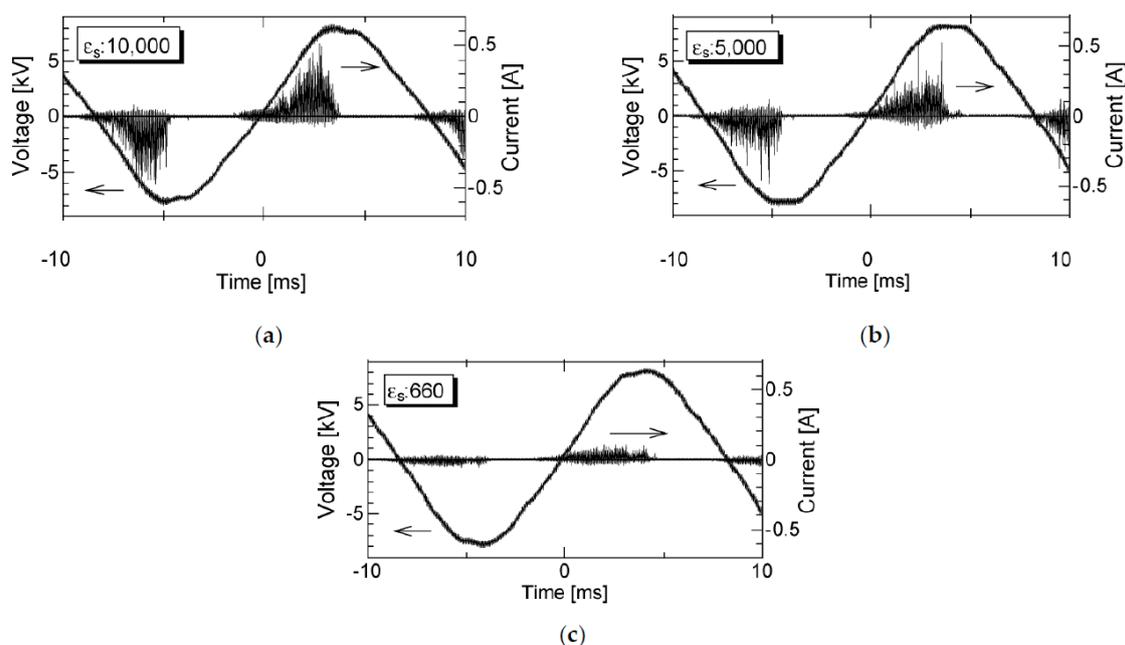
**Figure 4.** Waveforms of applied voltage and discharge current for different dielectric constant of spherical pellets (a)  $10^4$ ; (b) 5000 and (c) 650 (applied voltage = 14 kV; frequency = 60 Hz). Reprinted from [90]. Copyright (2016), with permission from IEEE.
