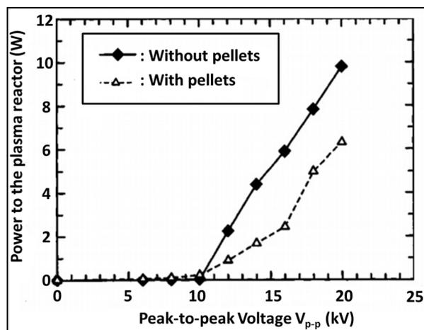
**Figure 3.** Effect of presence of packing material on the power to the plasma reactor (frequency of power supply = 60 Hz; packing material: BaTiO<sub>3</sub> pellets). Reprinted from [78]. Copyright (2016), with permission from IEEE.
