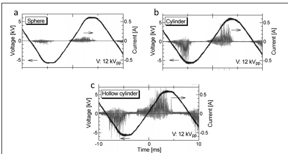
**Figure 6.** Waveforms of applied voltage and discharge current for different pellet shape such as (a) sphere; (b) cylinder and (c) hollow cylinder (packing material =  $\text{BaTiO}_3$ ; dielectric constant =  $10^4$ ; applied voltage = 12 kV; frequency = 60 Hz). Reprinted from [90]. Copyright (2016), with permission from IEEE.
