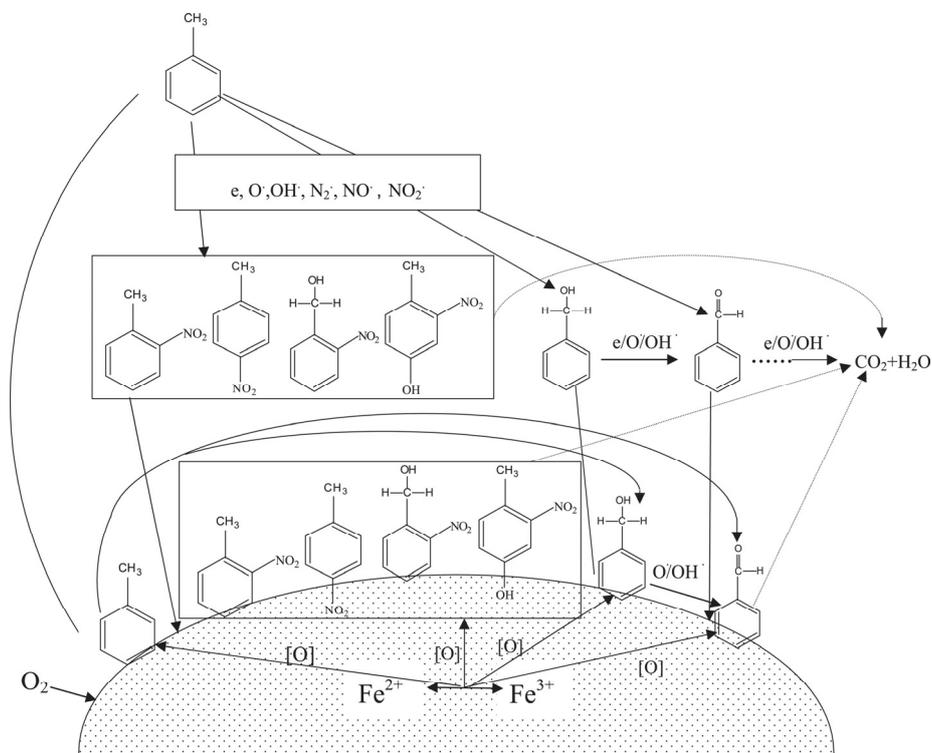
**Figure 7.** Pathways of toluene degradation in the gas phase and on the FeO<sub>x</sub>/SBA-15 surface. Reprinted from [116]. Copyright (2017), with permission from Elsevier.
