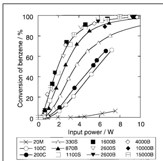
**Figure 5.** Effect of dielectric constant on the removal efficiency of benzene (Initial benzene concentration: 200 ppm; carrier gas: dry air; flow rate: 0.2 L/min; shape and size of the packing material: sphere of  $\phi$ 2 mm, numbers in legend box refer to dielectric constant value, M = Mg<sub>2</sub>TiO<sub>4</sub>, C = CaTiO<sub>3</sub>, S = SrTiO<sub>3</sub>, B = BaTiO<sub>3</sub>). Reprinted from [86]. Copyright (2016), with permission from IEEE.
