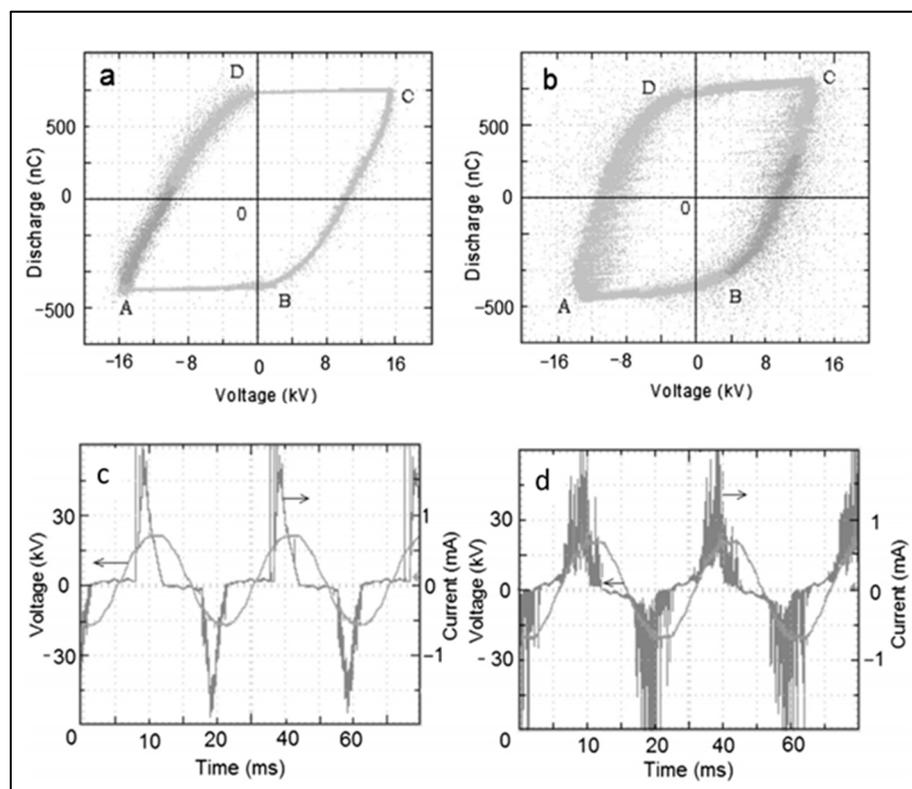
**Figure 2.** V-Q Lissajous figure in the (a) absence and (b) presence of ceramic Raschig rings (RR), voltage and current waveform in the (c) absence and (d) presence of ceramic Raschig rings (RR) at applied voltage of 12 kV (50 Hz and sine wave). Reprinted from [63]. Copyright (2016), with permission from Elsevier.
