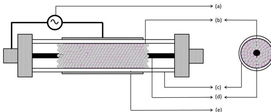
**Figure 1.** Schematic diagram of packed bed non-thermal plasma reactor and its cross-sectional view (a) Power source; (b) Packing material in discharge gap; (c) Dielectric barrier; (d) High voltage (or powered electrode) and (e) Ground electrode.
