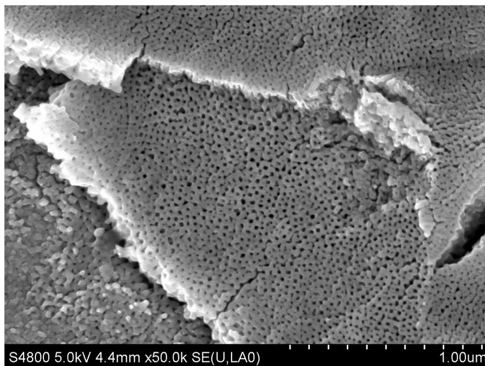
**Figure S6.** FE-SEM image of the nanoporous oxide layer.
