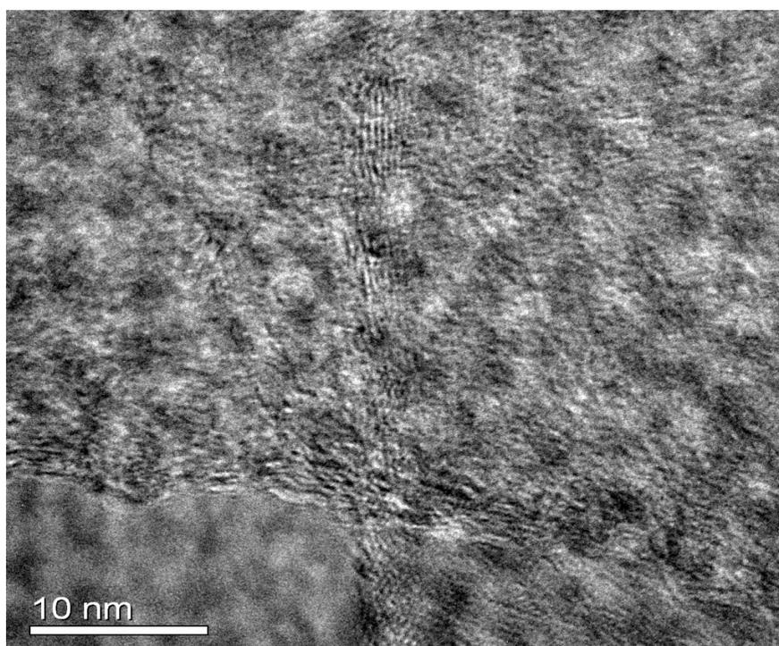
**Figure S20. HRTEM images of prepared graphene.** The graphene was no more than 7 layers thick.
