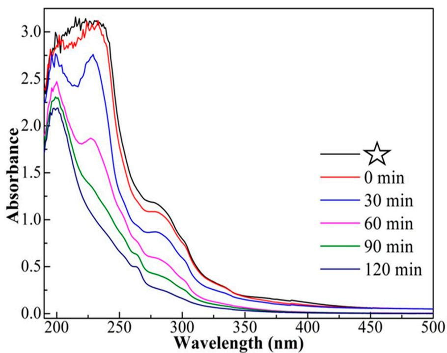
**Figure S18.** UV-Vis absorbance of the printing and dyeing wastewater during the photoelectrochemical degradation process. ☆ represents the absorbance of the waste water after flocculation and precipitation.
