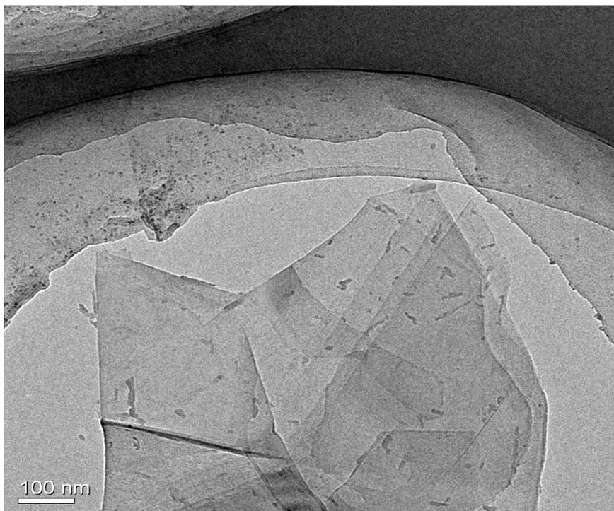
**Figure S19. TEM images of prepared graphene.** The as-prepared graphene was almost completely transparent and had an average length and width of about 500 and 300 nm.
