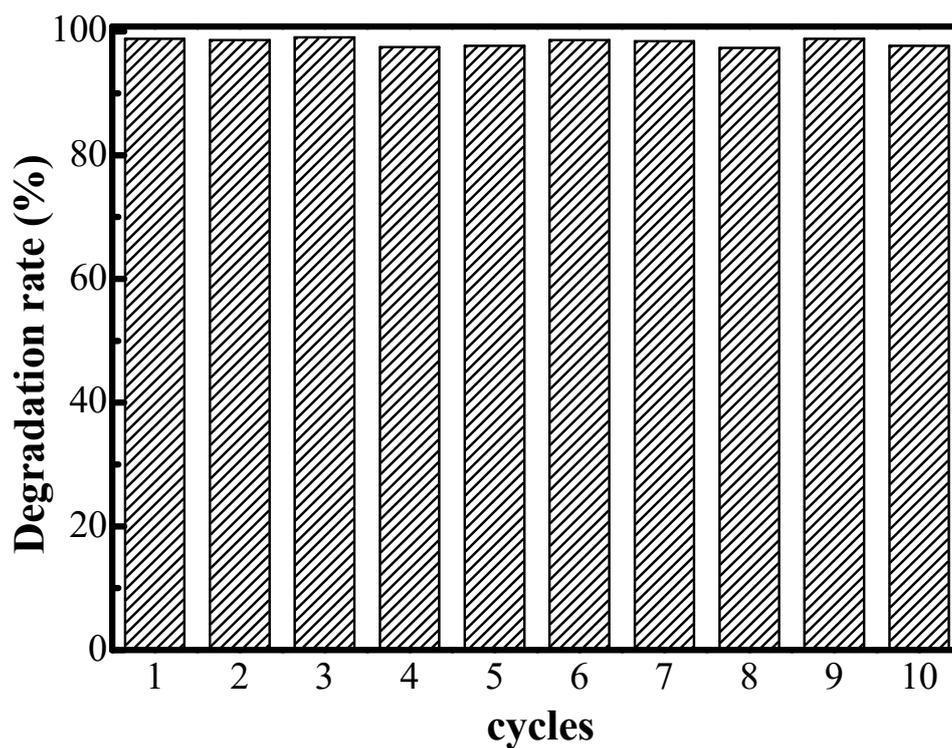
**Figure S16.** Stability test of methyl orange degradation for ten cycles under natural sunlight ( $C_{MO} = 20 \text{ mg L}^{-1}$ ,  $V_{MO} = 40 \text{ mL}$ ).
