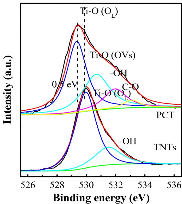
Figure S14. O 1s XPS spectra of the PCT film and TNTs.
