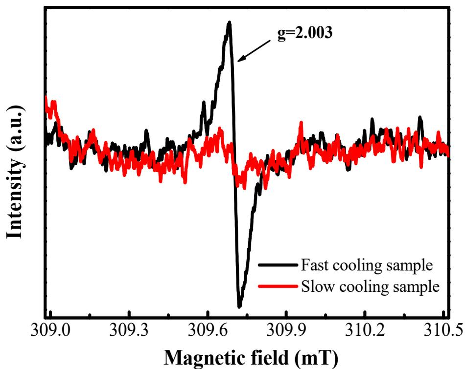
Figure S15. ESR spectra of PCT film with different cooling styles after calcination at 723 K for 2 h.
