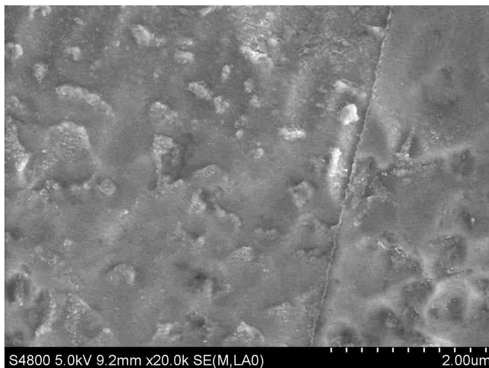
**Figure S2.** FE-SEM images of the TiO<sub>2</sub> film anodized in the electrolyte of magnesium nitrate solution (100 mg L<sup>-1</sup>, 50 mL) at 60 V for 2 min.
