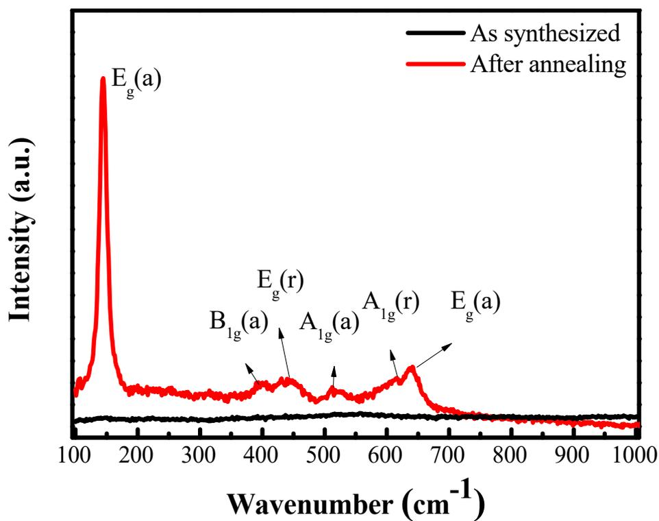
**Figure S10.** Raman scattering patterns of the PCT films, where the anatase and rutile vibration modes are labeled according to mode (a) and mode (r), respectively.
