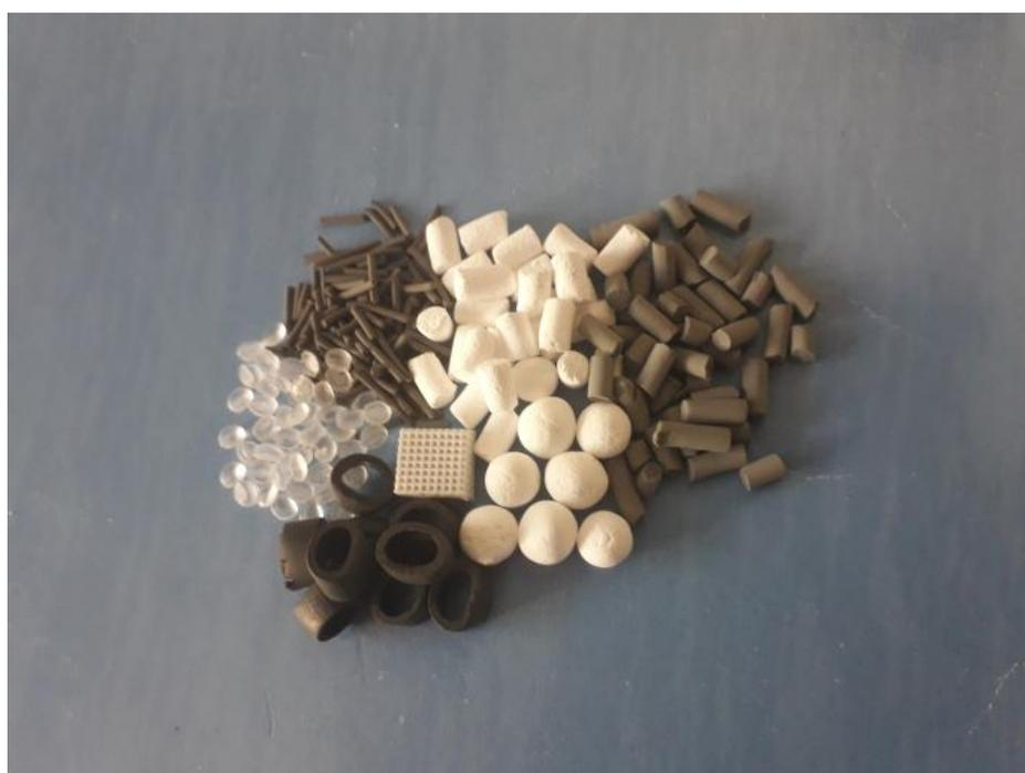
**Figure 3.** Different catalyst morphologies.
