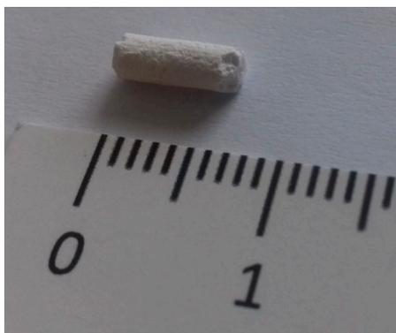
Figure 5. Homemade catalyst extrudate pellet.
