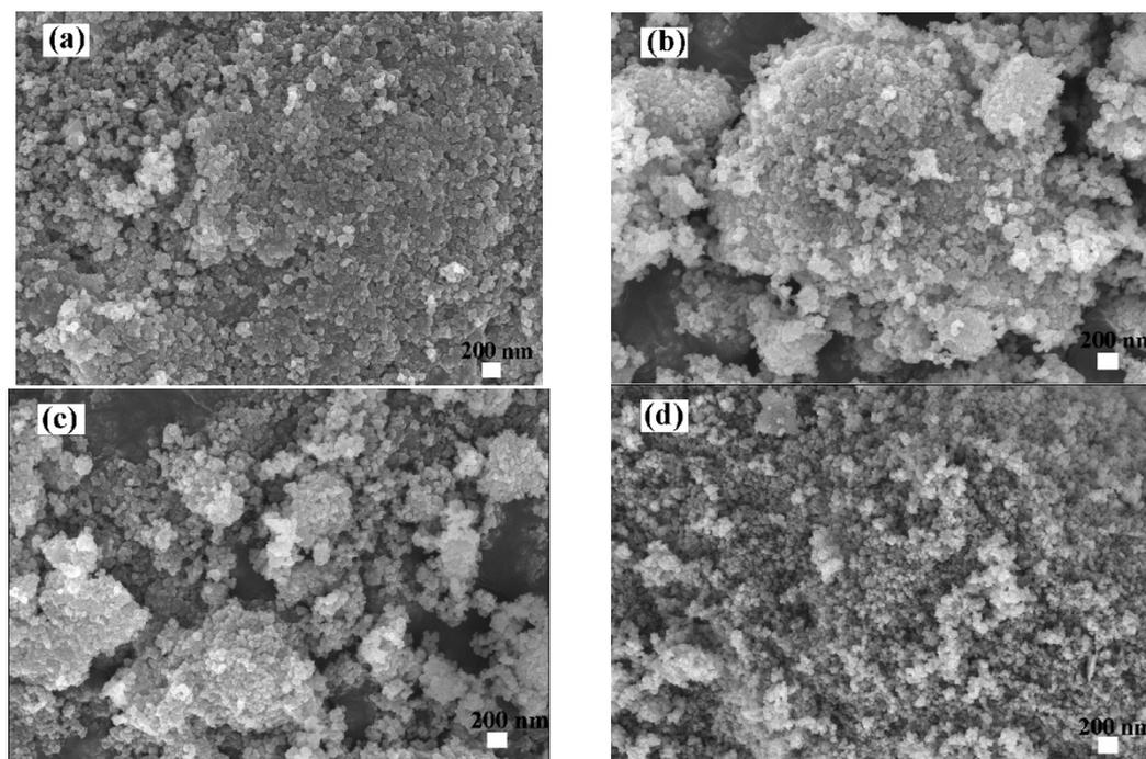
**Figure 3.** SEM micrograph for the catalysts: (a) 20%Ni/TiO<sub>2</sub>; (b) 10%Ni-10%Co/TiO<sub>2</sub>; (c) 10%Ni-10%Co/TiO<sub>2</sub>-A and (d) 20%Co/TiO<sub>2</sub> in different views.
