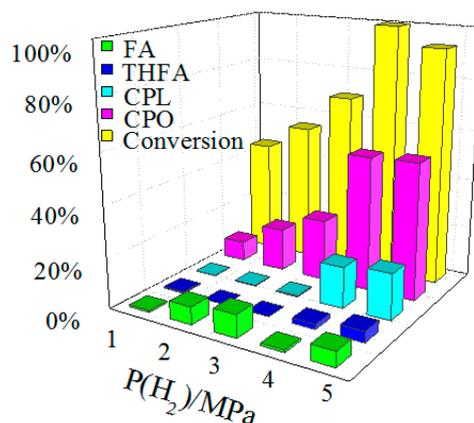
**Figure 5.** Conversion of furfural over 10%Co-10%Ni-TiO<sub>2</sub> at different H<sub>2</sub> pressure. Reaction conditions: FFA (0.5 g), catalyst (0.3 g), water (15 mL), 150 °C, 4 h.
