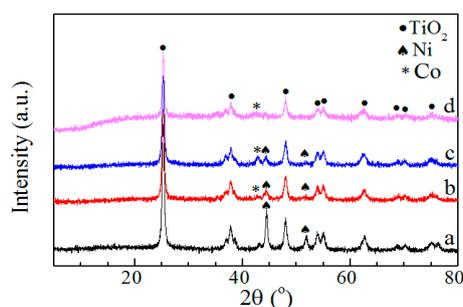
**Figure 1.** XRD patterns of (a) 20%Ni-TiO<sub>2</sub>; (b) 10%Co-10%Ni-TiO<sub>2</sub>; (c) 10%Co-10%Ni-TiO<sub>2</sub>-A; and (d) 20%Co-TiO<sub>2</sub> after reduction.
