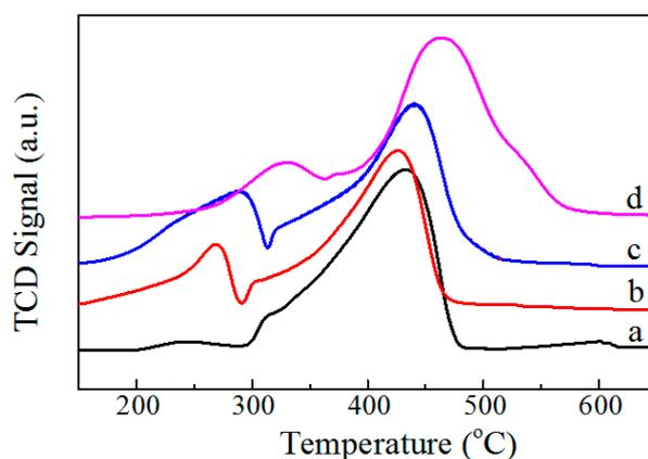
**Figure 2.** H<sub>2</sub>-TPR profiles of catalysts: (a) 20%Ni-TiO<sub>2</sub>, (b) 10%Co-10%Ni-TiO<sub>2</sub>, (c) 10%Co-10%Ni-TiO<sub>2</sub>-A, (d) 20%Co-TiO<sub>2</sub>.
