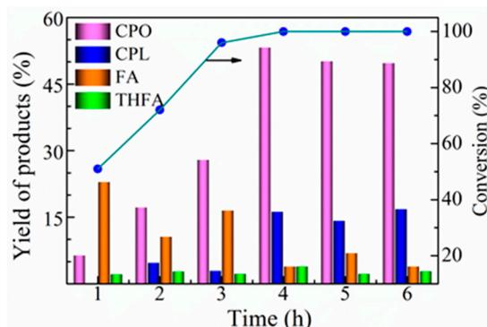
**Figure 6.** Effect of reaction time on FFA conversion and product selectivity over 10%Co-10%Ni-TiO<sub>2</sub>. Reaction conditions: FFA (0.5 g), catalyst (0.3 g), water (15 mL), 150 °C, 4 MPa H<sub>2</sub> (●: conversion).
