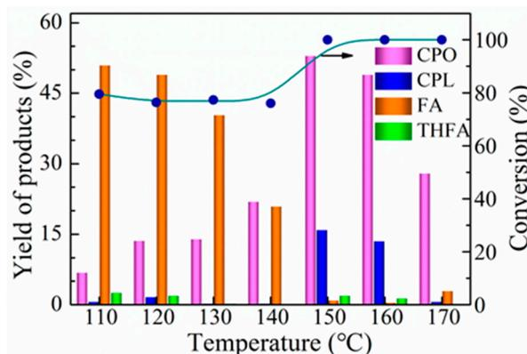
**Figure 4.** Conversion of furfural over 10%Co-10%Ni-TiO<sub>2</sub> at different temperatures. Reaction conditions: FFA (0.5 g), catalyst (0.3 g), water (15 mL), 4 MPa H<sub>2</sub>, 4 h (●: conversion).
