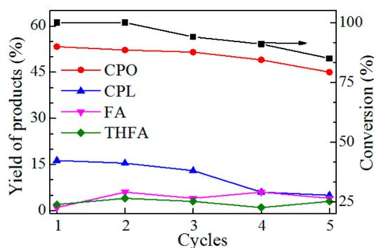
**Figure 7.** Reuse of the 10%Co-10%Ni-TiO<sub>2</sub> catalyst in FFA hydrogenation. Reaction conditions: FFA (5 mmol), catalyst (0.3 g), water (15 mL), 150 °C, 4 MPa H<sub>2</sub>, 4 h (■: conversion).
