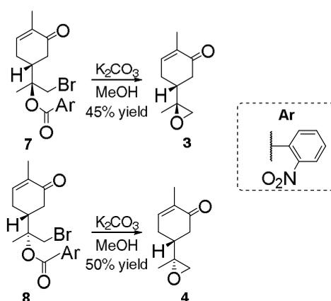
Scheme 2. Synthesis of 7,8-carvone epoxides **3** and **4**. Further research using *S*-carvone is in process in order to test the possible match–mismatch diastereoselectivity.
