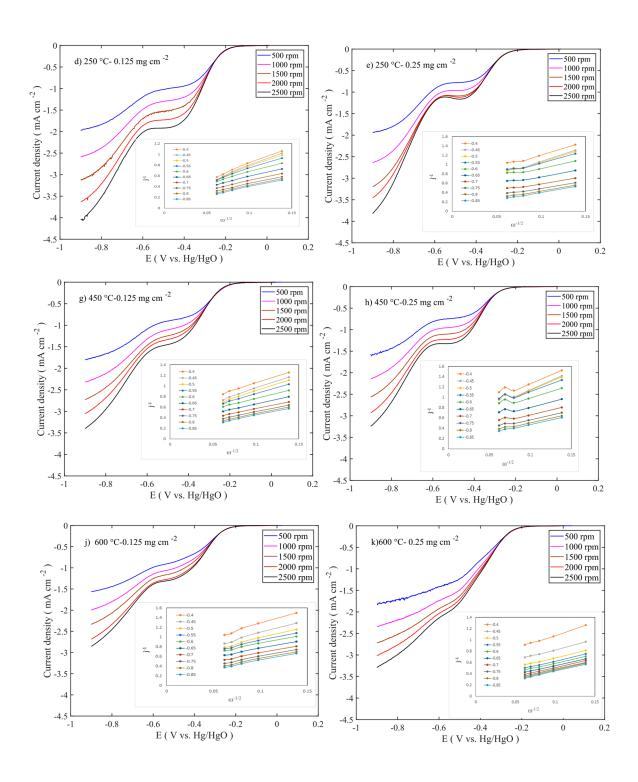
Figure S3. Electrochemical stability of Ni Fe oxide calcined at different temperature with three different mass loadings
