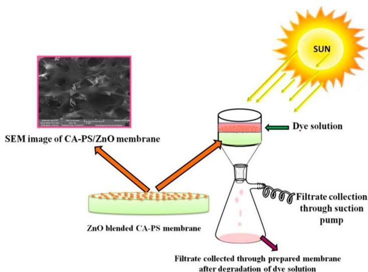
**Figure 8.** Schematic representation of the photocatalytic degradation of organic dyes over CA-PS-ZnO membrane. Reproduced by permission of Elsevier from [106].
