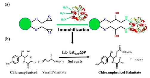
**Scheme 1.** (a)  $\text{Est}_{\text{BAS}}\Delta\text{SP}$  immobilization on epoxy resin Lx-105s and (b) the application of immobilized  $\text{Est}_{\text{BAS}}\Delta\text{SP}$  in the regioselective synthesis of chloramphenicol palmitate.
