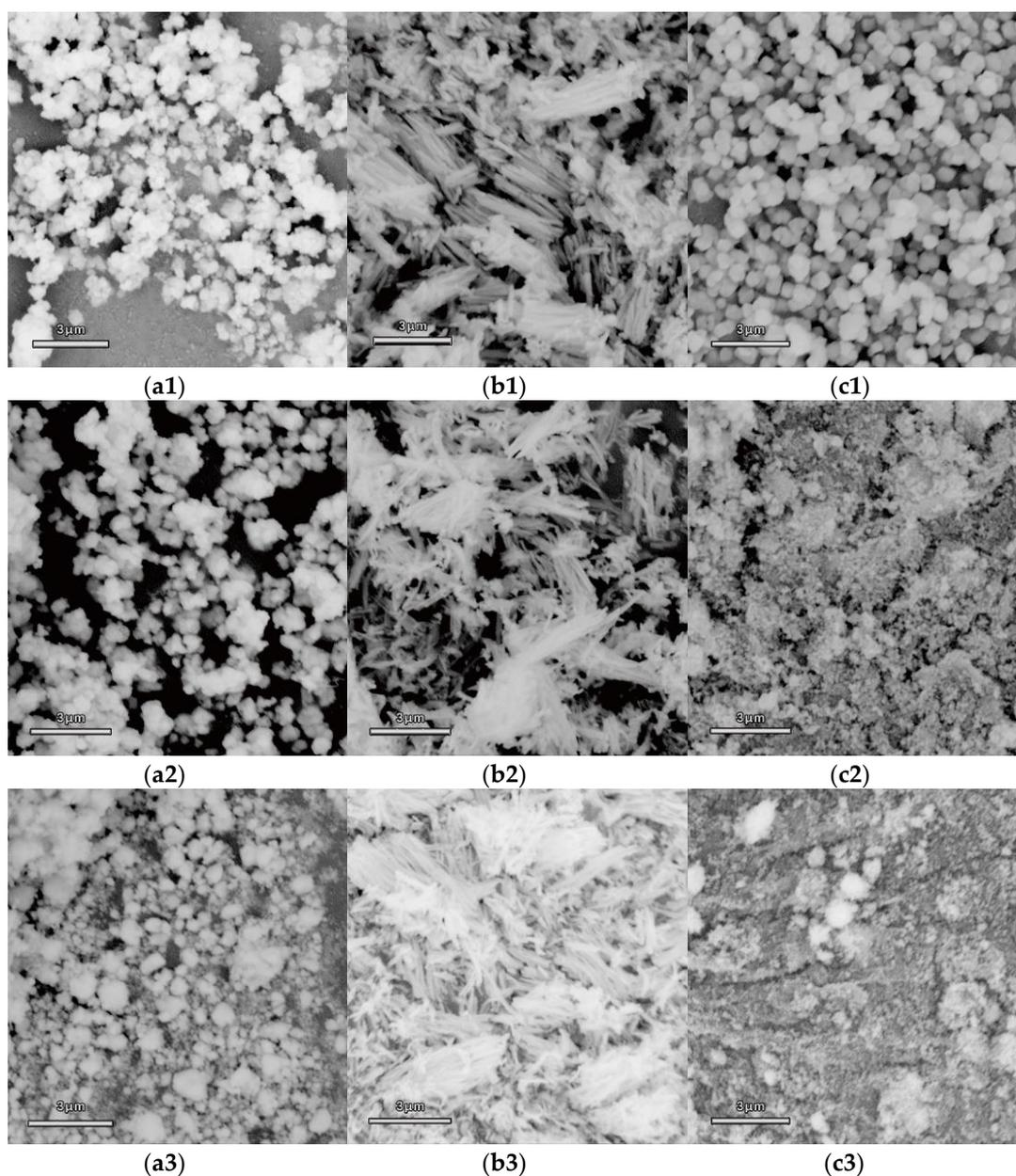
**Figure S1.** SEM images of Ce-MOF-808, Ce-BTC and Ce-UiO-66 before calcination (a1, b1, c1), Ce-MOF-808-250, Ce-BTC-340 and Ce-UiO-66-320 after calcination at 250 °C, 340 °C and 320 °C respectively (a2, b2, c2) and the corresponding CeO<sub>2</sub>-MOFs finally after calcination at 500 °C (a3, b3, c3).
