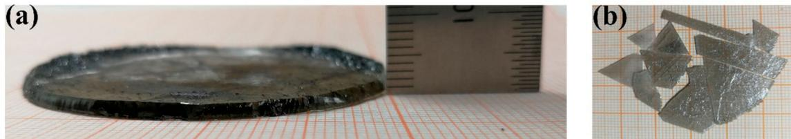
**Figure 7.** (a) Digital camera image of the freestanding GaN crystal produced using three-step process; (b) vestigial substrate.
