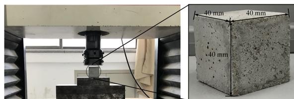
**Figure 2.** Setup of the uniaxial compression test.
