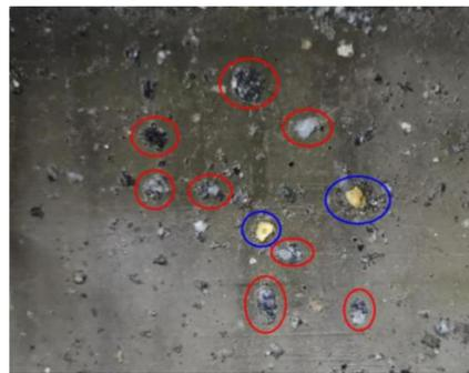
**Figure 7.** Typical photo for damage of aggregate in specimen FIG2A1-2 (red circle: coarse aggregate; blue circle: fine aggregate).
