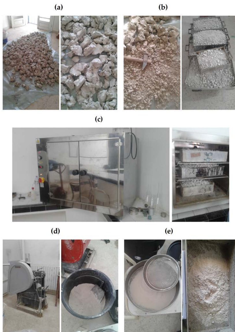
Figure 2. Different steps of marble powder preparation: (a) Air drying of marble sludge, (b) Crushing of marble sludge, (c) Drying of marble sludge in oven, (d) Grinding of marble sludge, (e) Sieving of marble powder.
