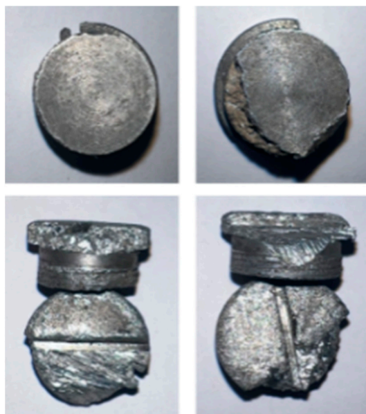
Figure 22. Wreckages of 14 mm alloy plug after fast cook-off.
