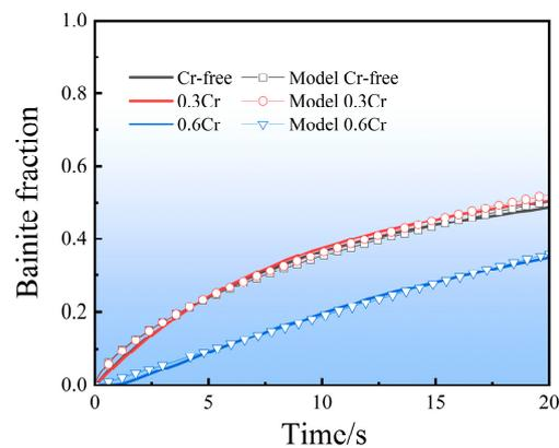
**Figure 7.** Kinetics of bainitic transformation of three experimental steels at 460 °C for 20 s.
