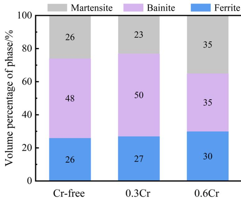
**Figure 6.** Volume fraction of the phases in three experimental steels after the isothermal process at 460 °C for 20 s.
