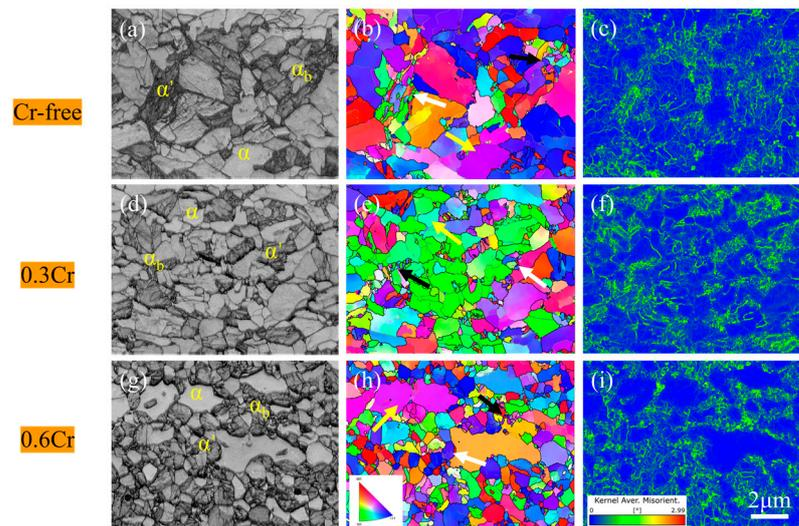
**Figure 4.** EBSD maps of three experimental steels: (a,d,g) band slope maps, (b,e,h) IPF color maps, and (c,f,i) KAM maps.  $\alpha$ : ferrite;  $\alpha'$ : martensite;  $\alpha_b$ : bainite. black arrow: bainite; white arrow: martensite; yellow arrow: ferrite.
