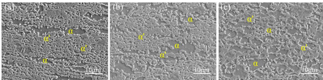
**Figure 2.** Microstructure of three experimental steels after Process 1. (a) Cr-free steel; (b) 0.3Cr steel; (c) 0.6Cr steel.  $\alpha$ : ferrite;  $\alpha'$ : martensite.
