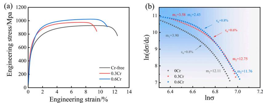
**Figure 8.** (a) Engineering stress–strain curves; (b) the modified C–J analysis of in  $\ln(d\sigma/d\varepsilon)$  vs.  $\ln(\sigma)$ .
