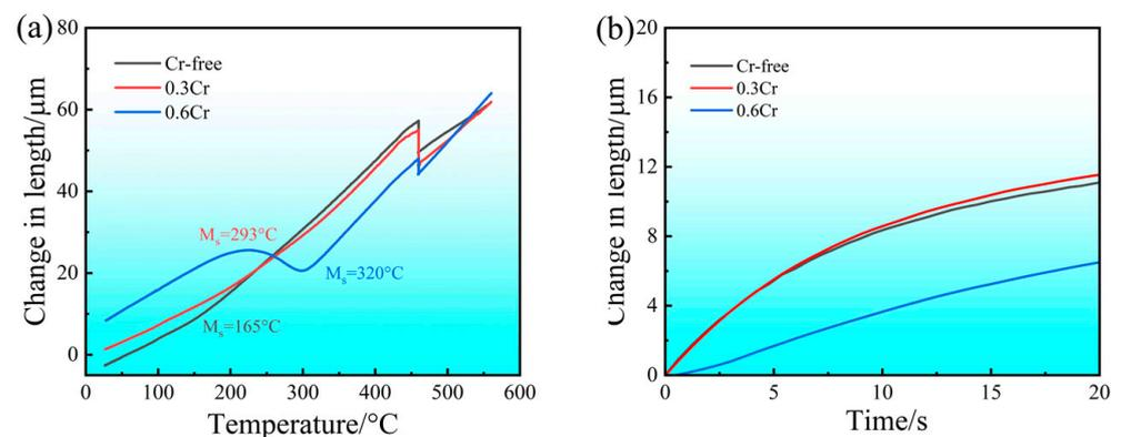
**Figure 5.** Dilatometric results of three experimental steels during the hot-dip galvanization process. (a) dilatation as a function of temperature; (b) dilatation as a function of time.
