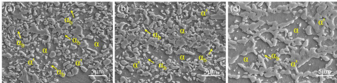
**Figure 3.** Microstructure of three experimental steels under the Process 2. (a) Cr-free steel; (b) 0.3Cr steel; (c) 0.6Cr steel.  $\alpha$ : ferrite;  $\alpha'$ : martensite;  $\alpha_b$ : bainite.
