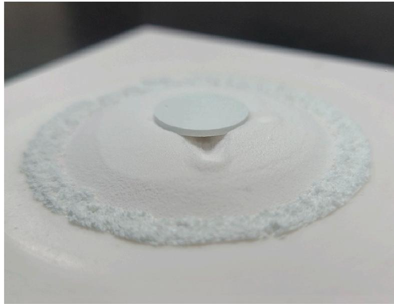
**Figure 9.** Pre-sintering samples that created a 0.5 cm wide tunnel.
