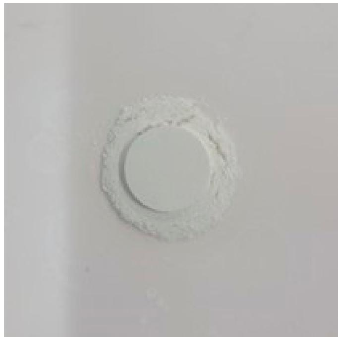
**Figure 5.** Image of sample in the setup after sintering while in contact with the mother powder.
