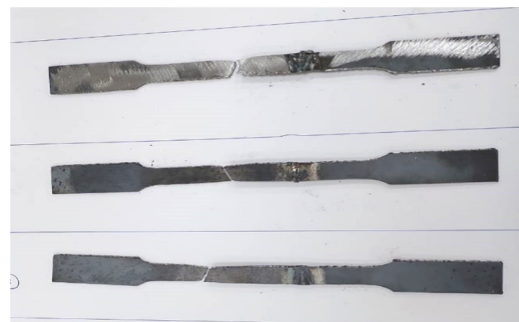
Figure 11. Tensile specimen for beads performed with an E 6013 electrode after breaking.
