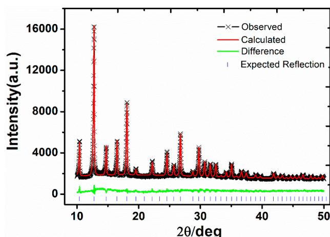
**Figure S1.** The powder X-ray diffraction (PXRD) spectra of MAF-7 refined by Le Bail method. The black and red symbols, and the purple continuous lines are experimental, calculated, and difference profiles, respectively, and the vertical markers indicate the allowed Bragg reflections.  $R_p = 5.0\%$ ,  $R_{wp} = 7.4\%$  and  $GOF = 4.598$ .
