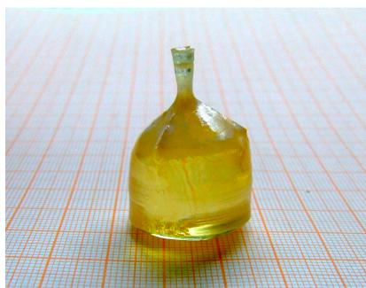
**Figure 1.** Photograph of the as-grown Mg:<sup>7</sup>LiNbO<sub>3</sub> crystal.
